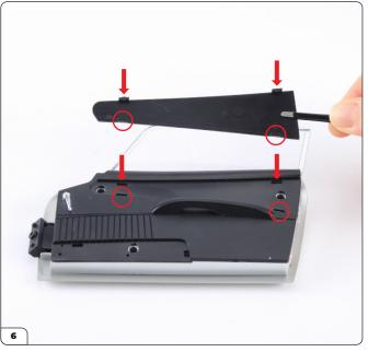
Align the top trim (7-D) with the recess in the door panel as shown. First fit the two tabs into the lower openings (circled), then push down firmly on the other tabs to press them into the two upper openings (arrows).
