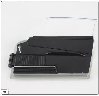
Press the bottom trim firmly into place, then align the L-shaped trim (7-B) with the three holes.
