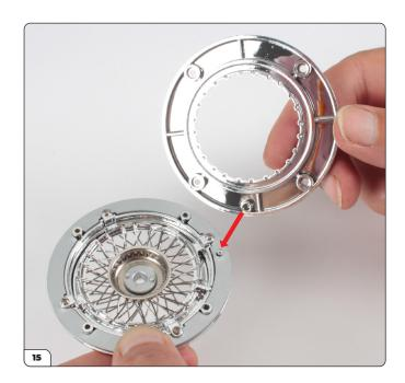
Align the inner wheel rim (3-A) with the assembly using the hole and pin as a guide.
