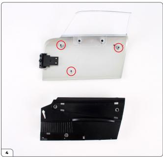
Fit the panel assembly onto the right door (stage 005) by pushing the holes over the posts (circled). Secure the panels using 3x DS02 screws.
