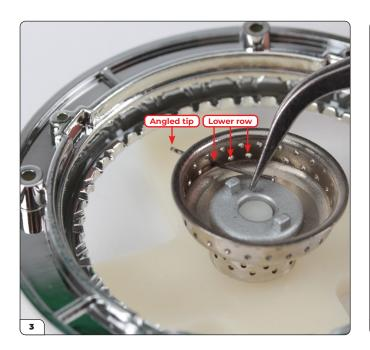
Open a bag of spokes (2-E) and thread the angled tip through one of the holes of the lower row.
