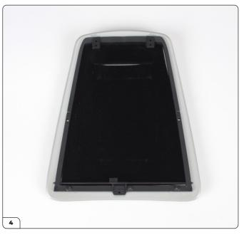
Fit the subframe in place on the bonnet, pressing firmly over the two pins highlighted in the previous step. Ensure the fit over these pins is flush.
