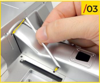
06/03 As you did in stage 05, join the support bar to the floor by orientating the pieces as shown in the photo. The longer angled end must again be in the lower position.
