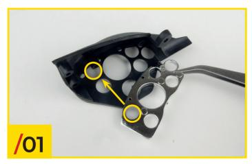
02/01 Position the frame on the inside of the dashboard as shown in the photo.
