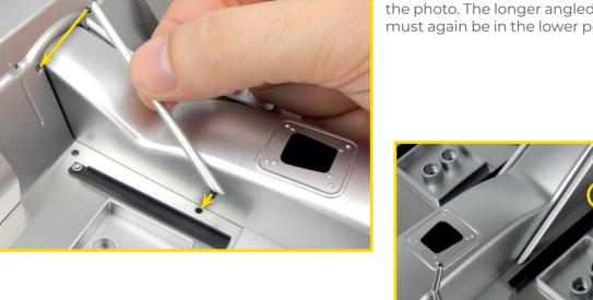
06/04 Insert three seat belt hooks received in stage 05 into their respective slots on the front floor. Note: the hooks have a D-shaped pin and the flat part of the pin should face towards the rear of your model.
