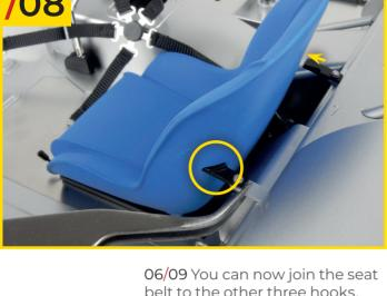
06/08 Insert the stoppers into the rear side of the seat.
