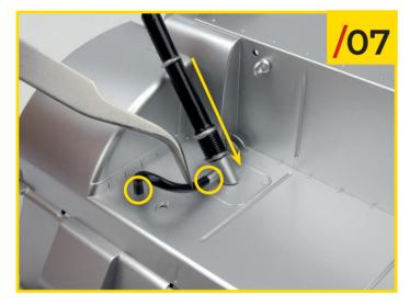
05/07 Join the oil filling pipe to the rear floor half, in the location you can see from the photo. Fit the ends of the hose onto the pins indicated.
