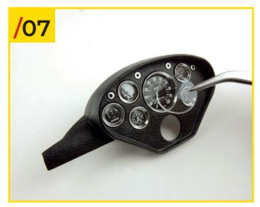
02/07 Now take the large lens and remove the films, as you did with the small ones in step 02. Insert the large lens into its recess on the outside of the frame.
