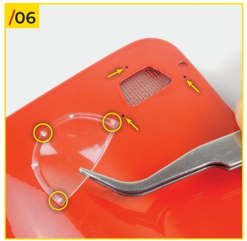
01/06 Using tweezers, install the left-hand air intake cover on the bonnet. You will notice that these pieces are not symmetrical: use the photo to match the pins on the underside of the left cover to the corresponding holes. Press lightly to fit the two pieces together.
