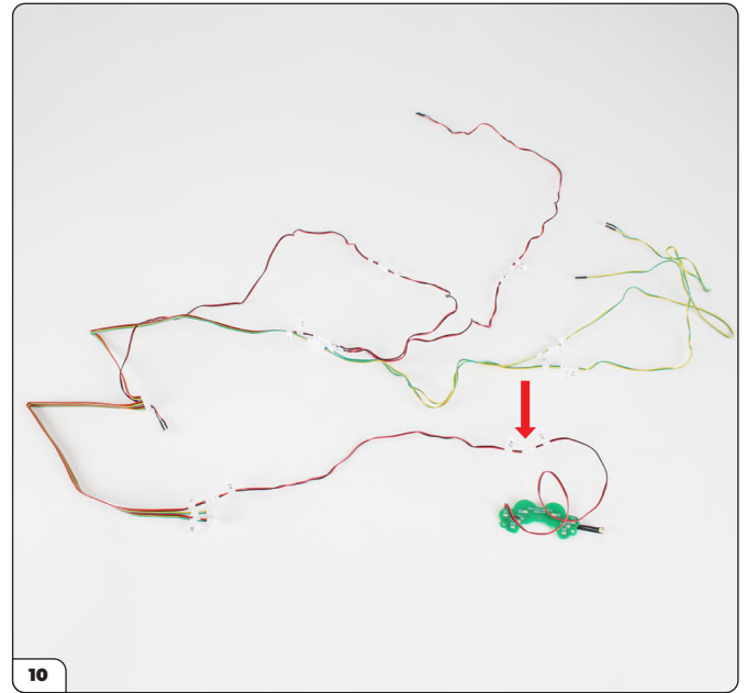
Plug LED cable 'A3' into its extension.
