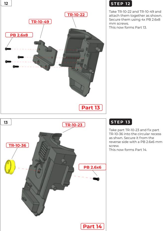
Take TR-10-22 and TR-10-49 and attach them together as shown. Secure them using 4x PB 2.6x8 mm screws. This now forms Part 13.
