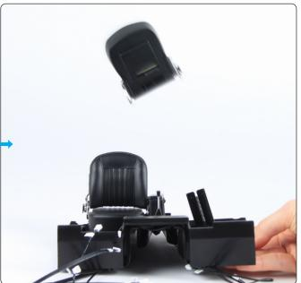
Place the assembly upright to test the ejector mechanism. Pull the lever to release the catch – the seat should shoot upwards at an angle.
