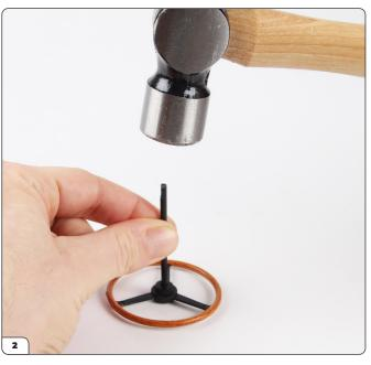
Carefully hammer the steering column into the steering wheel.
