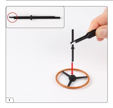
Take the steering column (57-B) and place the thin end without a hole (inset) into the shaped hole of the steering wheel (57-A).
