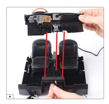
Take the cockpit floor assembly. Hold the instrument panel wire (marked '11') towards the front then align the dashboard assembly as shown.
