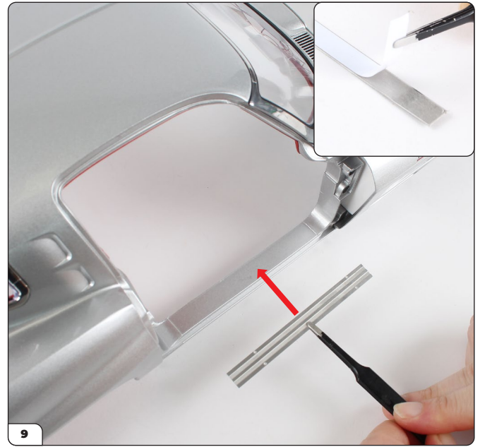
Peel the backing paper from one of the door sills (inset) then align it with the main body.
