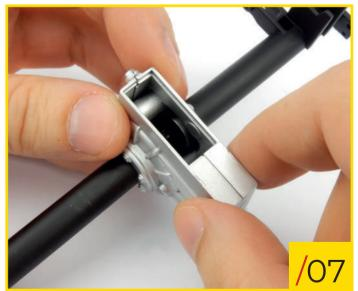
25/07 Bring the two halves of the differential housing together by sliding the left half towards the right half.
