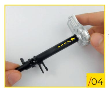
25/05 Fit the two axle shafts together. Orientate the pieces as shown and ensure the holes at the ends of the two half axle shafts line up.
