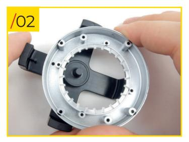
21/02 Insert the stud into the hole to fix the rim onto the jig. Before proceeding with the assembly, we recommend that you stick a small piece of double-sided sticky tape to the jig's central stud - this will help to hold the hubs in place. Alternatively, you can lay all the spokes in position and then dab a bead of glue on each one after stage 21/08.
