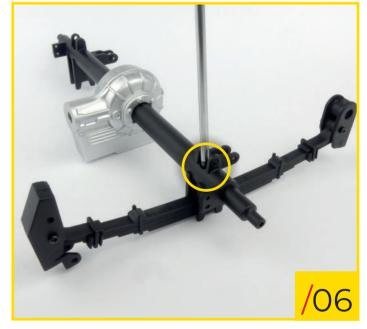
26/07 Turn the assembly over again and fit the central bracket into the position indicated in the photo. Ensure that the circled lug is oriented towards the rear end of the leaf spring.
