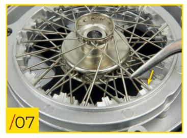
23/07 Place the straight end of the spoke onto the corresponding notch on the top level of the retainer ring. Repeat these steps for the other eleven type C spokes, until all the holes in the top row on the hub have been filled.
