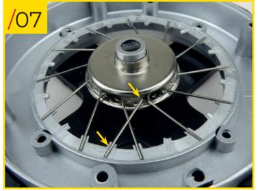
21/07 Now position the type A spokes (they are longer than the type B ones) by inserting their hooked end into the upper row of holes immediately to the left of the type B spokes, making sure they pass over the spokes inserted into the lower row of holes. Use the photo to help identify which notch you should position the other end of the spoke on. Always leave an empty hole between each spoke in the hub.
