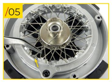
23/05 Place the straight end of the spoke on the notch on the lower level of the retainer ring as shown in the photo. Repeat these steps for the other eleven type C spokes, until all the holes in the lower row on the hub have been filled.
