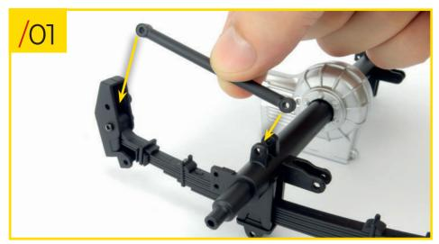
27/01 Retrieve the assembly you built in stage 26. Place one of the reaction struts onto the left rear leaf spring, as shown in the photo.
