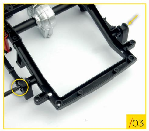
30/03 Secure the rear brackets to the chassis using two type B screws.
