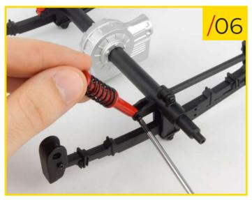
29/06 Secure the pieces together using a type G screw.
