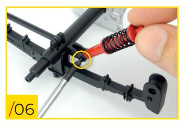
27/06 Secure the pieces together using a type G screw.
