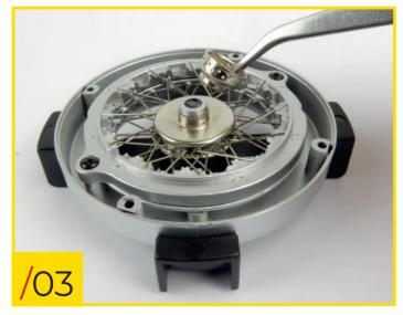
23/04 Insert the hooked end of one type C spoke into one of the holes in the lower row on the type C hub.
