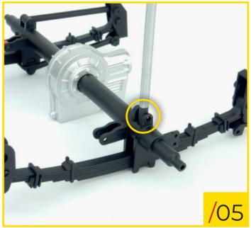
28/06 Turn the assembly over again and fit the central bracket into the position indicated in the photo. Ensure that the circled lug is oriented towards the rear end of the leaf spring.
