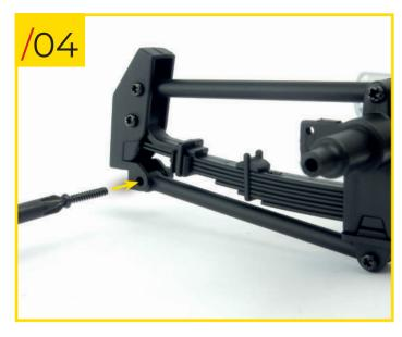
27/04 Secure the other end of the strut to the spring's front bracket using a type H screw.
