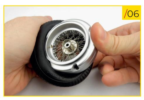
24/06 Slip the tyre onto the rim of the left front wheel.
