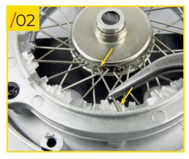
23/03 Once all the type A spokes have been added, position the type C hub that you received with stage 21 as shown in the photo.
