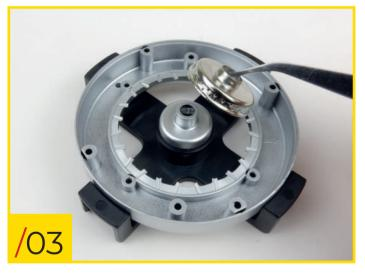
21/03 Place the type B hub onto the jig's central stud; once in place, press the type A hub on top of it, as shown in the photo.
