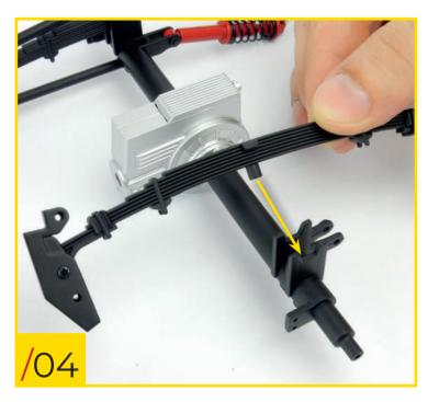
28/04 Retrieve the differential housing assembly and the rear axle shaft you assembled in previous stages. Orientate the pieces as shown and fit the leaf spring onto the right half of the axle shaft.
