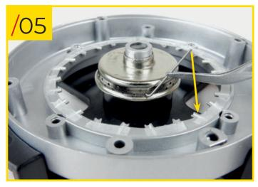
21/05 Position the type B spokes (they are shorter than the type A ones) by inserting their hooked end into the lower row of holes in the type A hub. Place the straight end of the spokes onto the corresponding notch on the edge of the rim (on the double-sided sticky tape). Always leave an empty hole between each spoke in the hub.
