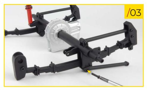
29/03 Position the second strut as shown and secure one end to the spring's central bracket by screwing a type G screw into the hole indicated.
