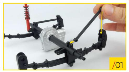
29/01 Retrieve the rear axle shaft you assembled in the previous sessions. Place one of the reaction struts onto the right rear leaf spring, as shown in the photo.
