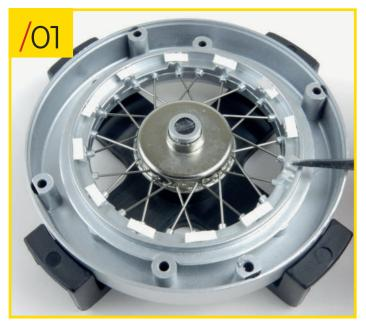
22/01 Place the left front wheel that you assembled in stage 21 on your workbench. Before proceeding with the assembly, we recommend that you stick small strips of double-sided sticky tape to the side edge of the spoke retainer ring 1. Alternatively, you can lay all the spokes in position and then dab a bead of glue on each one after stage 22/03.
