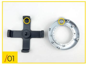
21/01 Place the jig and inner wheel rim on your workbench. The jig has a small fixing stud on it, this should be inserted into the corresponding hole in the rim.
