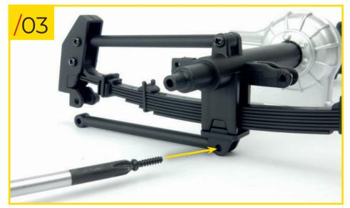
27/03 Position the second strut as shown and secure one end to the spring's central bracket by screwing a type G screw into the hole indicated.
