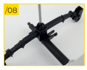
26/08 Secure the central bracket to the rest of the assembly using a type B screw.
