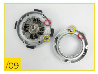
23/09 Fit the outer wheel rim to the rest of the wheel. To line up the holes, match up the arrows circled in red.
