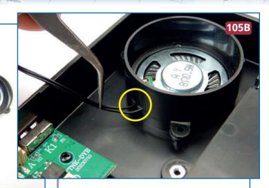
**2** Fit the speaker assembly into the battery box **104B**, so that the holes in the holder **105B** align with the raised screw sockets in the box **104B**. Note that the cables should run out of the holder on the side next to the circuit board. Fix in place with three **BP** screws.
