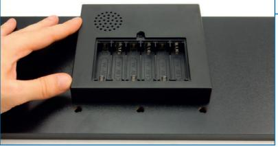
**5** Make sure that you do not pull any of the sockets out of the circuit board. Turn the battery box the right way up and position it on the stand so that the screw holes are aligned. Turn the stand upside down so that you can fix the battery box in place using four washer screws **105C** (circled, above).
