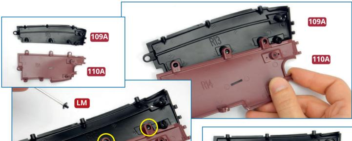
Take the hull sections **110A** and **109A** (supplied with the previous issue). Screw holes in tabs along the upper edge of part **110A** fit over raised screw sockets in part **109A**. Fix them together with three **LM** screws. You will need the Allen key supplied with **issue 15** to tighten the screws.
