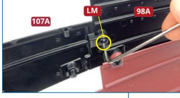
**2** Fix hull section **107A** in place with an **LM** screw. You will need to use the Allen key supplied with issue 15 to tighten the screw.
