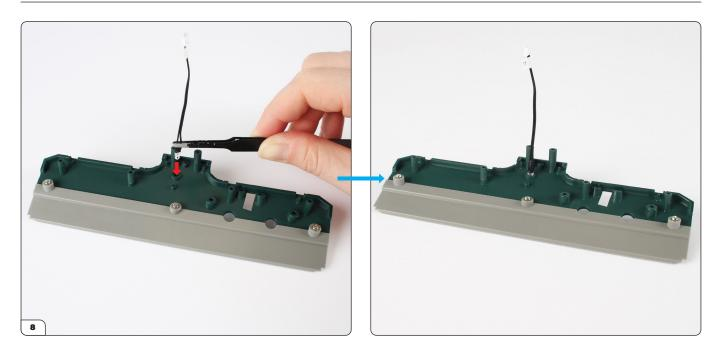
Take the radar LED cable No. 11 (37-E) and press the bulb into the hole.
