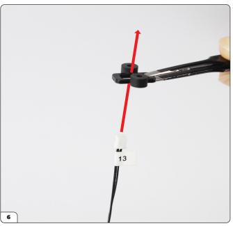
Put the power switch cable No. 13 plug (42-F) through the bracket (42-E). Make sure the bracket is oriented as shown.
