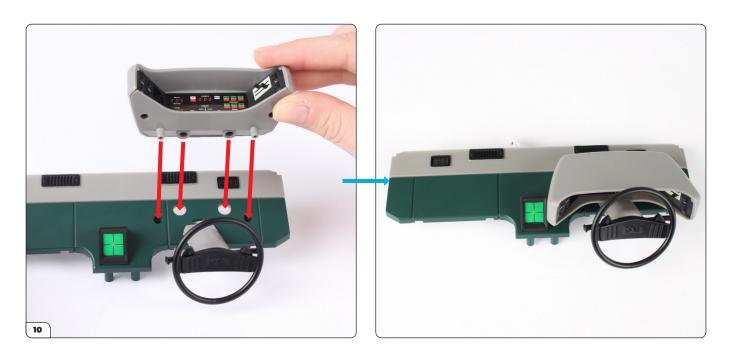
Push the instrument panel (stage 036) into the holes behind the steering wheel.
