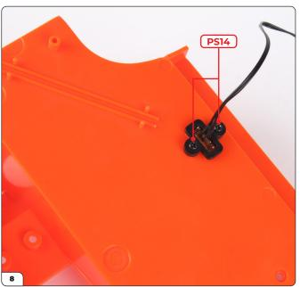
Secure the bracket to the floor using 2x PS14 screws.
