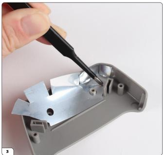
Remove the reflector sticker from the backing paper and press it firmly onto the instrument panel top.
