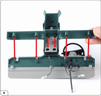
Position the centre console over the two middle screw posts, then align the dashboard bottom panel as shown.
