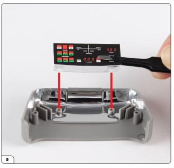
Place the centre display onto the screw posts.
