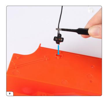
Move the bracket down the cable to the switch then push the switch into the rectangular opening on the bottom of the cockpit floor.
