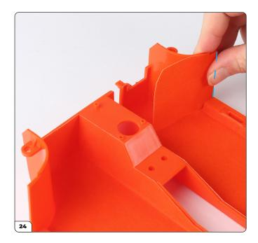
Press the sticker onto the right-hand side, aligning the outside edge first (dashed line).
