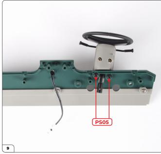
Place the steering column cover into the screw holes as shown.
