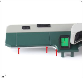
Press the trim firmly in place, making sure there are no gaps between the trim and the dashboard as shown in 3a.
