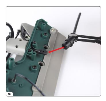
Push the drive shaft (38-B) onto the steering column.
