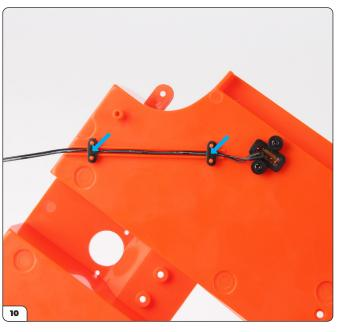
Secure the cables by pressing the two cable brackets (42-D) in place.
