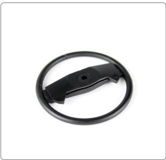
Take the crash pad (38-F) and press it into the back of the steering wheel (38-A).
