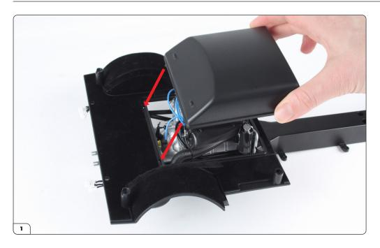
Align the engine cover (35-A) with the rear floor as shown. Push the two tabs into the corresponding holes.
