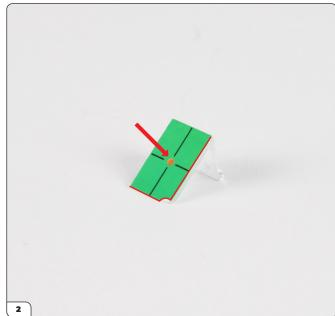
Take the radar glass (37-D) and radar sticker. Note the corner notches indicated by the red lines.
