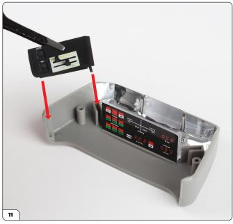
Push the right display into the instrument panel top.
