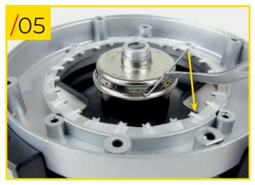
31/05 Install the type B spokes (they are shorter than the type A ones) by inserting their hooked end into the lower row of holes in the type A hub. Place the straight end of the spokes onto the corresponding notch on the edge of the rim (on the double-sided sticky tape). Always leave an empty hole between each spoke.
