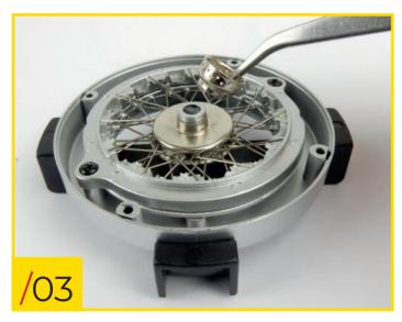
33/03 Once all the type A spokes have been added, position the type C hub that you received with stage 31 as shown in the photo.
