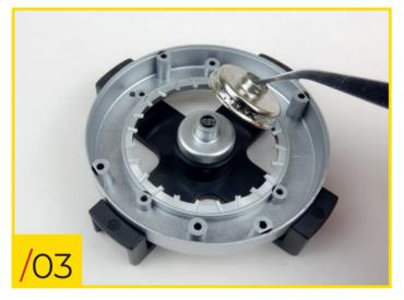
31/03 Place the type B hub onto the jig's central stud; once in place, place the type A hub on top of it, as shown in the photo.
