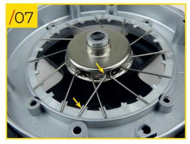
31/07 Now install the type A spokes (they are longer than the type B ones) by inserting their hooked end into the upper row of holes immediately to the left of the type B spokes, making sure they pass over the spokes inserted into the lower row of holes. Use the photo to help identify which notch you should position the other end of the spoke on. Always leave an empty hole between each spoke.
