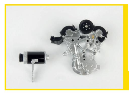
STAGE 40 IS COMPLETE Here's how the dynamo and timing chest look at the end of this assembly phase. Keep them in a safe place until needed.
