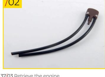
37/03 Retrieve the engine assembly and slide the other four long leads (stage 36) onto the studs on the right distributor cap.
