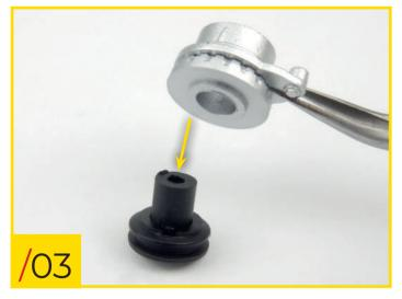
40/03 Insert the stud on the pulley into the hole in the support to fit the two pieces together.
