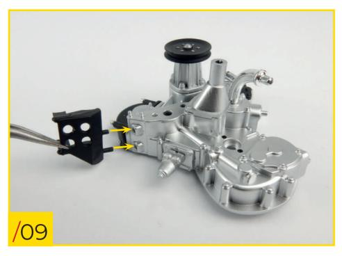
40/09 Fit the dynamo bracket to the timing chest that you assembled in the previous stages. Check the photo to make sure they are fitted together correctly.
