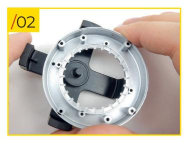
31/02 Insert the stud into the hole to fix the rim onto the jig. Before proceeding with the assembly, we recommend that you stick a small piece of double-sided sticky tape to the template's central stud - this will help to hold the hubs in place. Alternatively, you can lay all the spokes in position and then dab a bead of glue on each one after stage 31/08.
