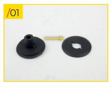
39/01 Fit the two parts of the pulley together, using the photo and the shape of the pieces as a guide.
