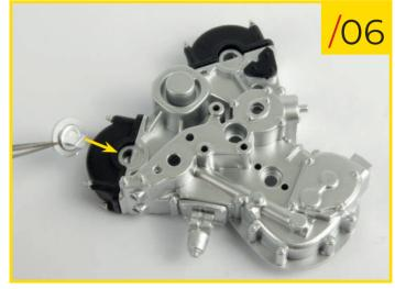
38/06 Place the right covering disk into its hole in the timing chest, as shown.
