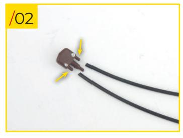
36/03 Retrieve the engine assembly and slide four long leads onto the studs on the left distributor cap.
