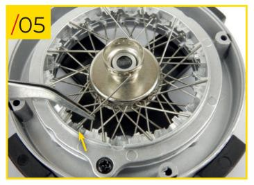
33/05 Use the photo to help put the straight end of the spoke on the notch on the lower level of the housing. Repeat these steps for the other eleven type C spokes, until all the holes in the lower row on the hub have been filled.
