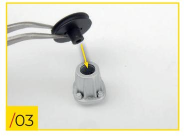
39/03 Fit the pulley to the pulley mount, as shown in the photo.
