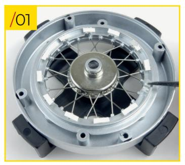
32/01 Place the right front wheel that you assembled in stage 31 on your work surface. Before proceeding, we recommend that you stick small strips of double-sided sticky tape to the side edge of the spoke retainer ring 1. Alternatively, you can lay all the spokes in position and then dab a bead of glue on each one after stage 32/03.
