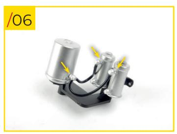
35/06 Fit the two filters to the pump support and insert the fittings into the holes in the components, as shown in the photo.
