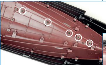
**2** Turn the hull right side up and fix the **PM** screws in place in the following order: first fit and tighten the three screws circled in yellow (top and top right); next, fit and tighten the five screws on the starboard side, circled in white (above); finally, fit and tighten the five screws on the port side circled in green (right).
