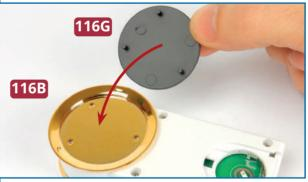
4 Position the rear rim of the telegraph 116B as shown, fitting the pegs on the back into holes in part 116A (above, left). Take part 116G and fit the pegs into the holes in part 116B (above). Slide the battery cover 116H into the hole in the back of part 116A.
