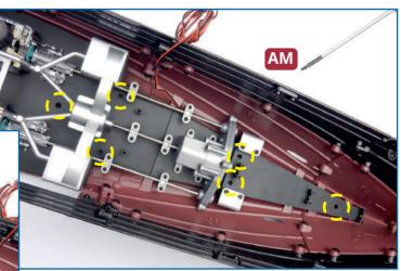
**3** Fix the engine assembly to the bottom of the hull using three **AP** screws and six **AM** screws. (The **AP** screws fix the deck beneath the reciprocating engines to the plastic section of the hull, left; the **AM** screws fix the engine room deck panels to the metal section of the hull, above.)
