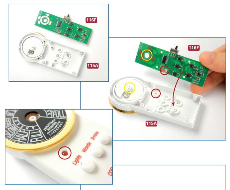
2 Position the circuit board 116F inside the front of the remote control 115A. Ensure that the red LED fits in the hole (circled in red) and the large hole fits on the peg in the centre of the part 115D (circled in yellow). Fix the board in place with four AP screws. Do not over tighten the screws as this may damage the circuit board.
