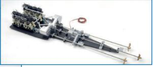
**1** Take the completed engine and propeller assembly from **issue 40**. Remove the plates **391**, **40F** and **40H**, as indicated (circled). Then remove the three propeller shafts. It is advisable to label the shafts (port, centre, starboard) so that you can replace them correctly.
