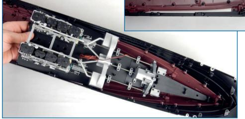
2 Now position the engine assembly inside the hull from **issue 113**, taking care to ensure that the screw holes in the engine room deck **36A** align with screw holes in the bottom of the hull (circled).
