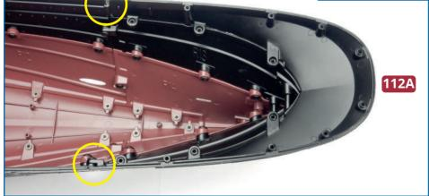
Take the hull assembly from the previous issue and the stern section **112A**. Fit part **112A** to the previous section as shown, checking that the tabs at each end of the stern section are fitted correctly (as circled in yellow, above and left).
