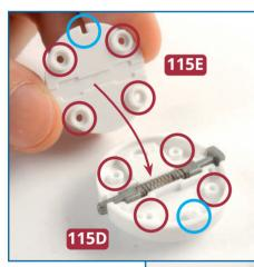
**4** Fit Disc B **115E** over Disc A **115D**. Check that the screw holes are aligned and the tab in part **115D** fits into the notch in part **115E** (circled in blue). Fix the discs together with four **KP** screws.
