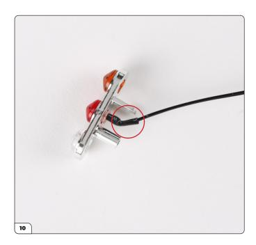
Carefully bend the wire away from the screw post as shown.
