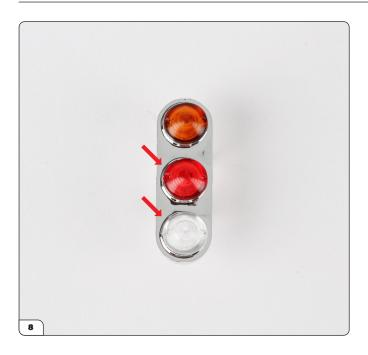
Press the red brake light (86-E) into the middle hole and the transparent reverse light (86-D) into the bottom hole.
