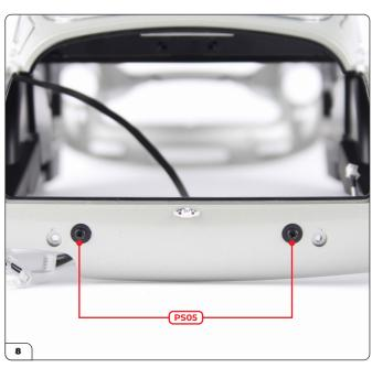
Secure using 2x PS05 screws.
