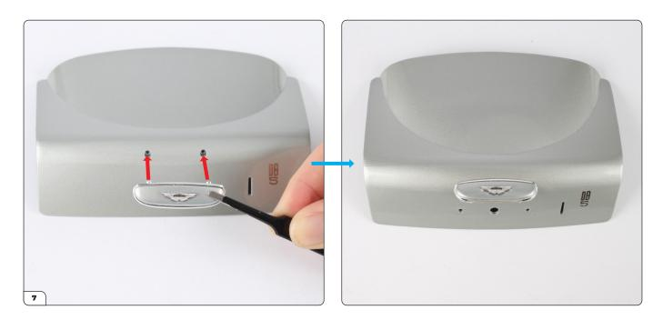
Take the rear number plate light assembly (stage 089) and press it into the two upper holes in the boot lid (stage 091).
