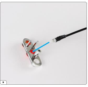
From the other side, push the brake light LED (86-G) into the brake light.
