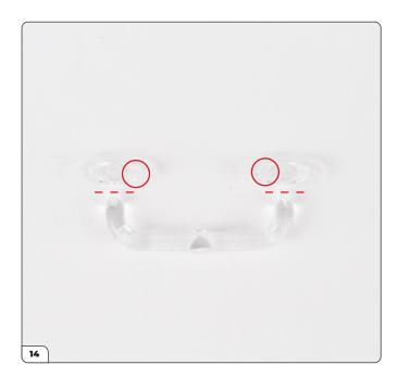
Take the sprue with the left (89-I) and right (89-J) rear number plate light. The parts are marked with "L" and "R" (circled). Cut the lights from the sprue at the point marked with a dashed line.
