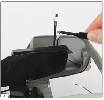
Place the main body upside down on your work surface. Fit the wire plug (No. 13) through the rectangular hole in the wheel arch as shown.
