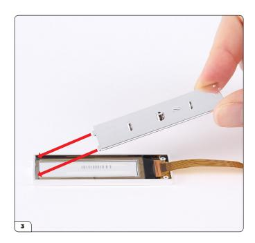
Place the screen into the frame, then align the frame back (92-B) with the assembly.
