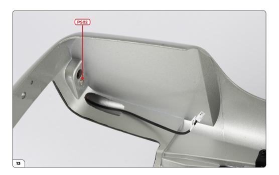
Secure from inside the main body using a PS02 screw.
