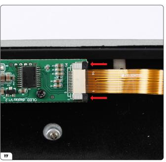
Lock the socket by pushing the black section back in.
