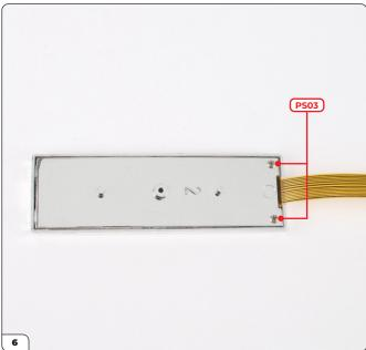
Turn the number plate over and check the screen is centred (dashed line). Carefully adjust the position by sliding the screen if needed.
