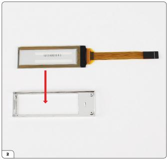
Align the screen with the rear number plate frame front (92-A) as shown.
