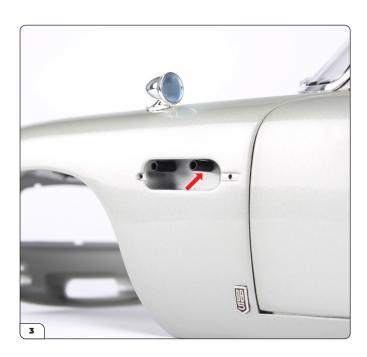
Take the remaining casing ejector port and press it firmly into the other hole.
