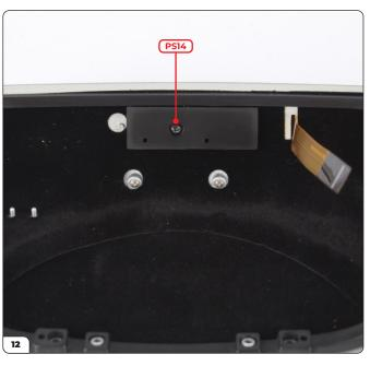
Secure the circuit board mount and the number plate with a PS14 screw.
