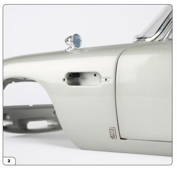
Push the casing ejector port firmly into the hole.
