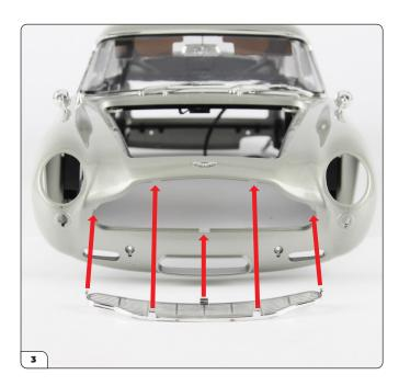
The front grille (91-B) fits into the front of the main body using five clips (arrows).
