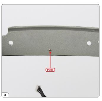
Secure the latch with a PS03 screw.
