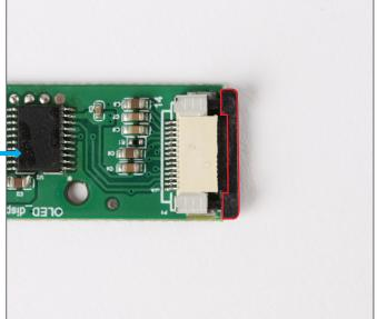
Take the circuit board (92-C) and unlock the socket by sliding the black section out as shown.
