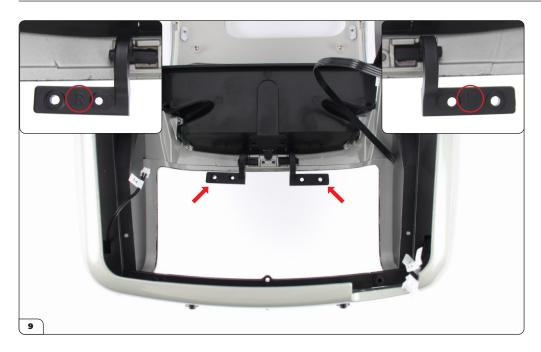
Take the right (89-F) and left (89-E) boot hinges. Position them on the main body as shown. The parts are marked with "R" and "L" (inset images).
