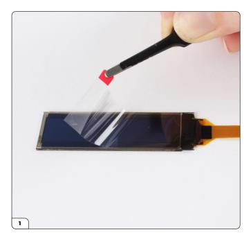
Take the rear number plate screen (92-E) and peel the protective film from it.
