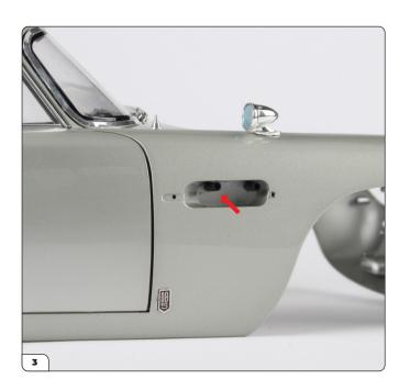
Take the remaining casing ejector port and press it firmly into the other hole.
