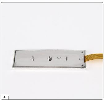
Fit the back in place. You may need to adjust the position of the screen slightly to allow the front and back to fit together.
