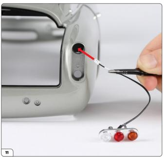
Fit the plug through the top hole in the rear right recess on the main body.
