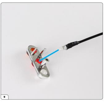
From the other side, push the brake light LED (85-G) into the brake light.
