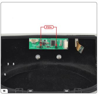
Position the circuit board over the two screw holes then secure it in place with 2x PS14 screws.
