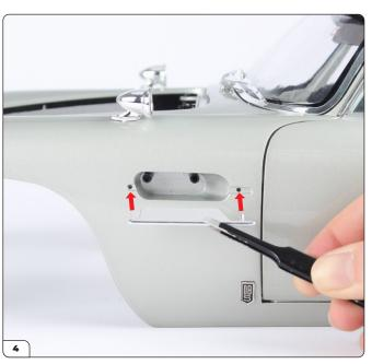
Align the side strake (85-A) with the main body as shown.
