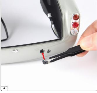
Turn the assembly over and secure the frame to the rear wheel arches with 2x PS05 screws.
