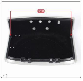
Fit the boot lid frame then secure with 2x DS06 screws.
