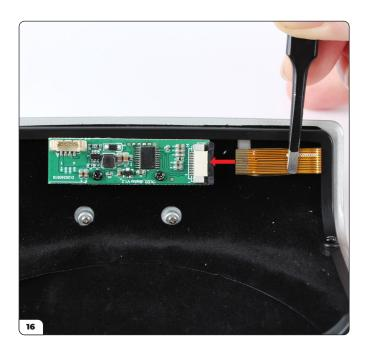
Push the ribbon cable into the unlocked socket.
