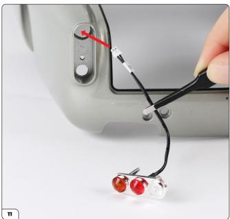
Fit the plug through the top hole in the rear left recess on the main body.
