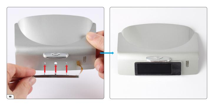
Align the rear number plate with the boot lid and press it in place, pushing the ribbon cable through at the same time. Make sure the pins and screw post are fully inserted into the holes for the next step.
