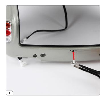
Place the main body assembly on your work surface. Press the boot latch (89-G) into the three holes. The latch can only fit in one orientation.
