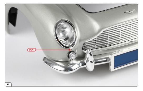
Screw the bezel to the main body with a DS41 screw.
