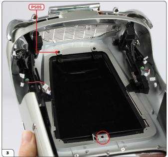
Close the bonnet, making sure the bonnet lock goes into the hole (circled). Screw a PS05 screw halfway into the other hinge. Tighten both screws firmly once you are happy with the placement of the bonnet.
