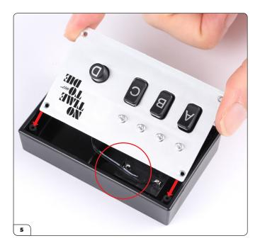
Place the remote control front onto the body. Make sure the wire does not get trapped (circled).
