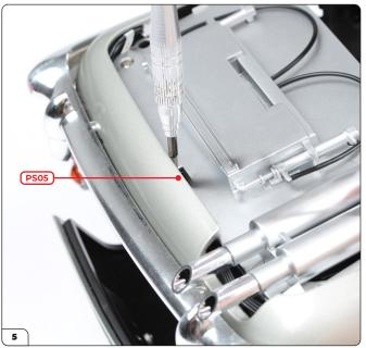
Screw a PS05 screw into the back of the chassis.
