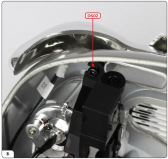
Screw the mechanism to the second screw post with a DS02 screw.
