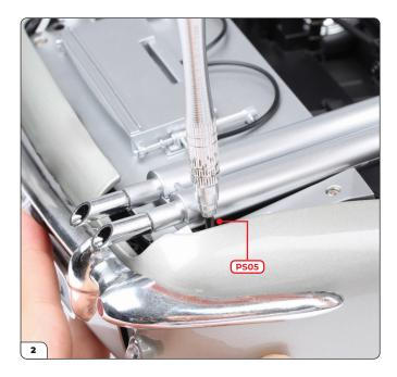
Screw a PS05 screw into the rear left corner.
