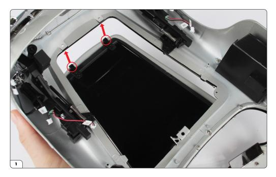
Place the main body (stage 099) upside down on your work surface. Align the bonnet (stage 001) with the main body. Check that the hinge joints (circled) are pointing upwards, then push them into place.
