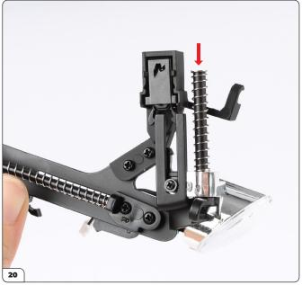
Place the short spring (96-J) onto the headlight shaft.
