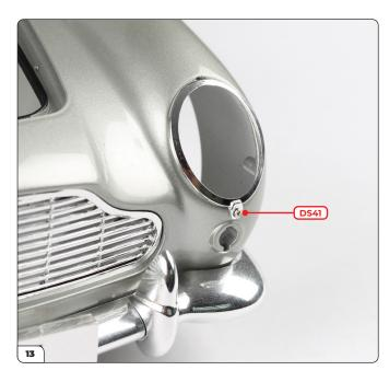
Screw the bezel to the main body with a DS41 screw. Be very careful your screwdriver doesn't slip and scratch the paintwork!
