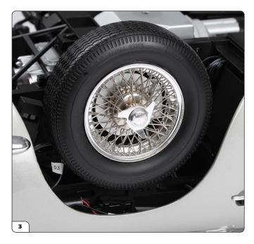
Place the hub cap (stage 004) onto the wheel. The magnet will hold it in place.
