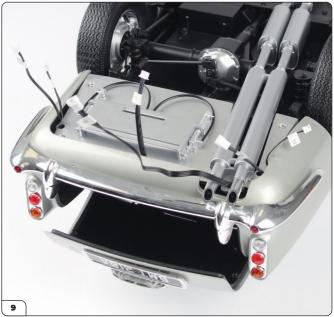
While applying pressure, lower the rear end of the chassis into the body. Make sure the screw hole highlighted in the previous step doesn't damage the body.
