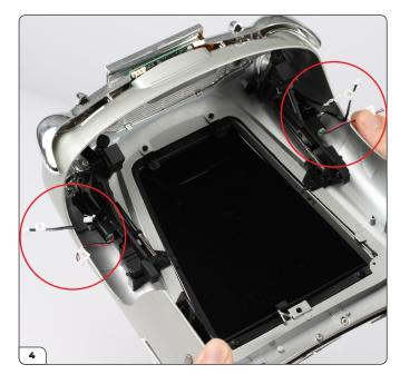
Bend the wires at the front over the wheel arches.
