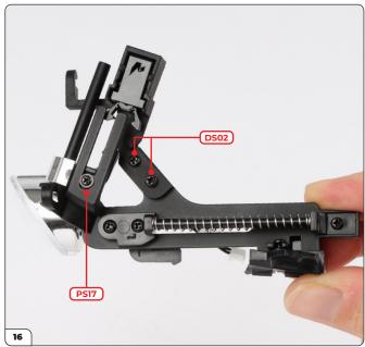
Screw the parts together with 2x DS02 screws. Screw the headlight stopper with a PS17 screw.
