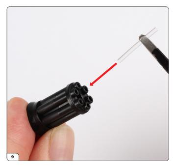
Take one of the light rods (95-K) and push it into a barrel.
