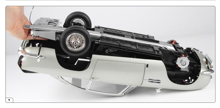
Carefully lower the front of the chassis into the main body.
