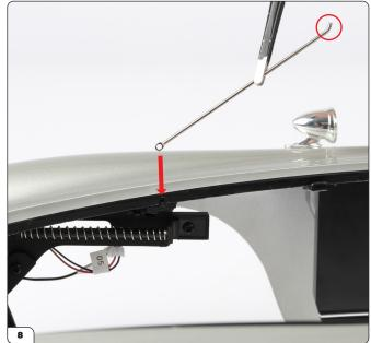
Align one of the bonnet struts (99-A) with the main body as shown. Make sure the end (circled) is pointing upwards.
