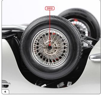
Push the other wheel (stage 029) onto the front left hub and screw in a DS12 screw.
