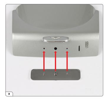
Push the rear number plate (100-F) into the boot lid. The pins are different sizes to ensure the correct orientation.
