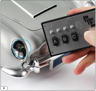
Press the headlights in and the miniguns out. Press the "D" button to start the minigun motor. The barrels will also illuminate from the LED. Press the button again to turn them off.
