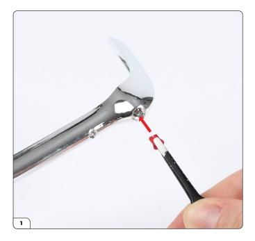
Push one of the rear bumper reflectors (93-D) into the rear bumper (93-A). The reflector is shaped so it will only go in one way.
