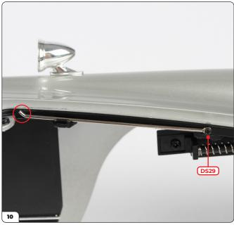
Screw the second bonnet strut to the main body with a DS29 screw in the same way.
