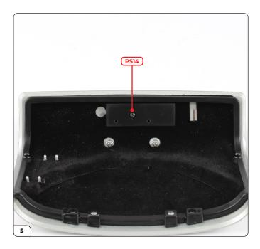
Screw the circuit board mount to the rear number plate with a PS14 screw (stage 092).
