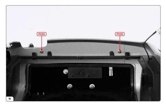
Screw the rear bumper to the body with 2x PS20 screws.
