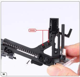
Screw the parts together with 2x DS02 screws.
