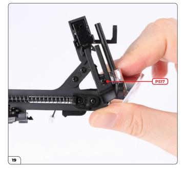
Screw the headlight stopper with a PS17 screw. Don't overtighten as the part should be able to slide up and down the rail.
