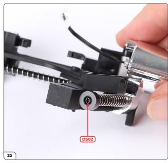
Screw the cap to the shaft with a DS02 screw.
