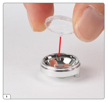
Press the headlight glass (95-C) into the reflector (95-B). There is a small tab which goes into a small recess (arrow).
