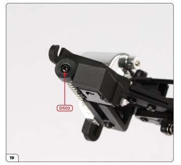
Screw the cap to the shaft with a DS02 screw.
