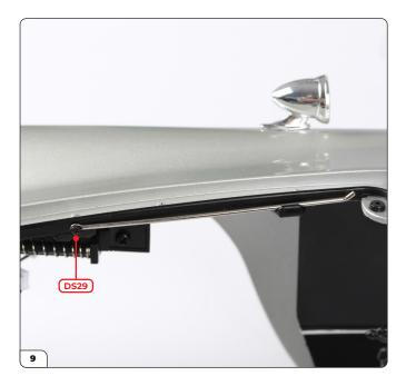
Screw the bonnet strut to the main body with a DS29 screw.
