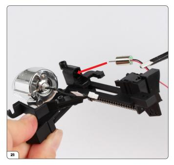
Push the motor (98-L) into the minigun stopper.
