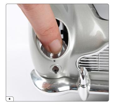
Push down on the headlight to release it from the clamp.
