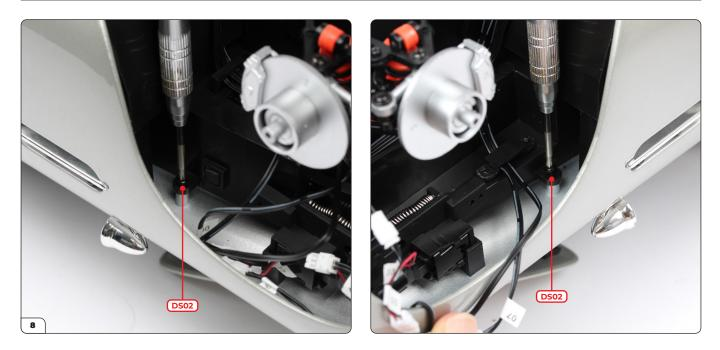
Screw 2x DS02 screws into the two holes in the front wheel arches.
