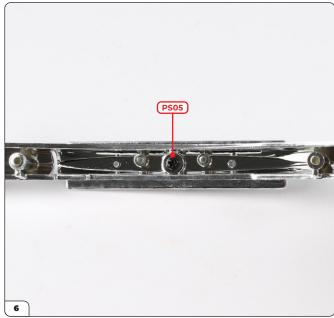
Screw the front number plate to the front bumper with a PS05 screw.
