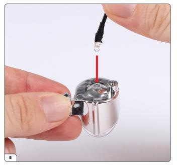
Gently push the headlight LED (95-L) into the headlight housing.
