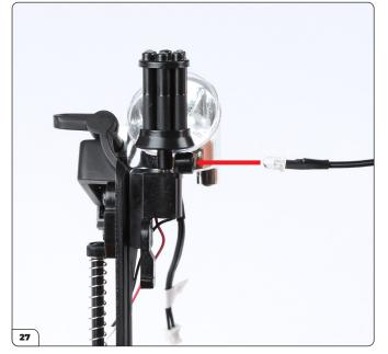
Push the muzzle flash LED (96-M) into the minigun stopper.
