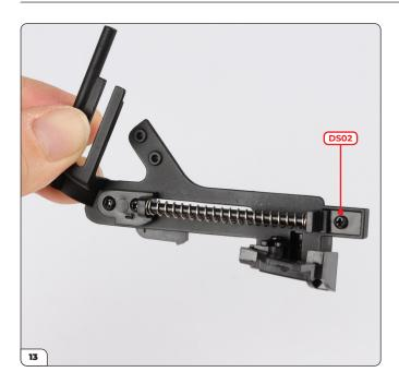
Push the other end of the shaft into the recess and screw it in using a DS02 screw.
