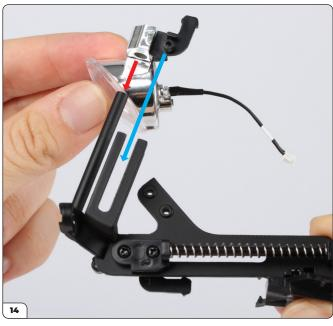
Push the left headlight housing onto part 1, fitting the headlight stopper between the rails as shown by the blue arrow.
