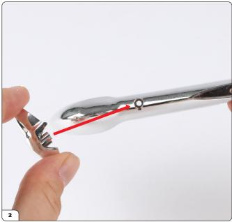
Push the front right overrider into the front bumper (94-A). Make sure you are placing it on the correct side.
