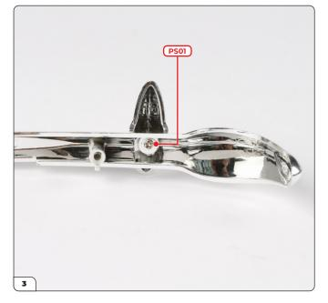
Screw the overrider to the front bumper with a PS01 screw.
