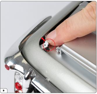
Tuck the cables at the rear of the model into the gaps between the body and the chassis.
