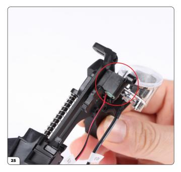
Press the motor firmly in place, taking care not to damage the wires.
