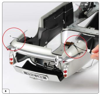
Bend the wires at the rear over the body.
