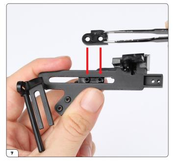
Hold the minigun stopper in place and turn the assembly over. Place the minigun stopper bracket (96-E) over the screw holes in the orientation shown.
