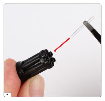
Take one of the light rods (97-K) and push it into a barrel.
