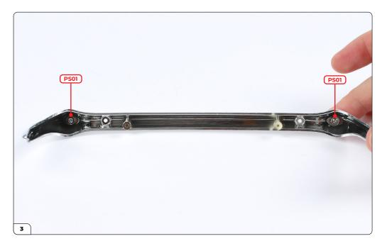
Screw the reflectors to the rear bumper with 2x PS01 screws.
