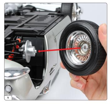
**Finishing the Model** Push the wheel (stage 004) onto the front right hub.
