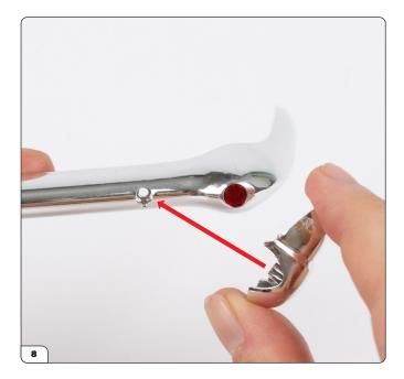
Take the rear right overrider (93-C) marked with "R R". Push it into the rear bumper.
