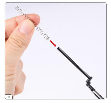
Place the long spring (96-K) onto the shaft (96-I).
