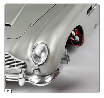
Tuck the cables at the front of the model into the wheel arches.
