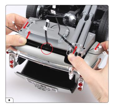
Note the screw hole (circled) at the rear of the chassis. Push the end of the chassis with your thumbs while pulling the rear wheel arches in the opposite direction (arrows).
