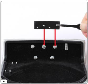
Align the circuit board mount (stage 092) with the inside of the boot lid. Press it onto the screw post and pin.
