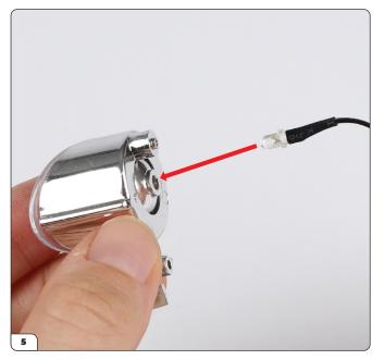
Push the headlight LED (97-L) into the headlight housing.
