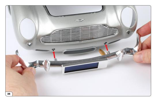
Push the front bumper into the main body (stage 93).
