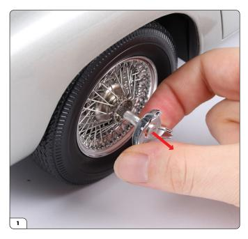
**Installing the Slim-line Tyre Slashers** Pull the tyre slasher and hub cap out from the rear wheel.
