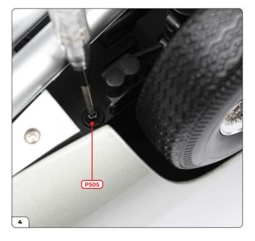
Screw a PS05 screw into the hole behind the rear left wheel.
