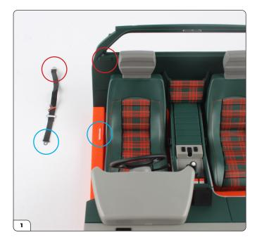
Take the cockpit assembly (stage 048). When fitting the seat belts, the longer end fits into the bulkhead and the shorter end fits into the cockpit floor.
