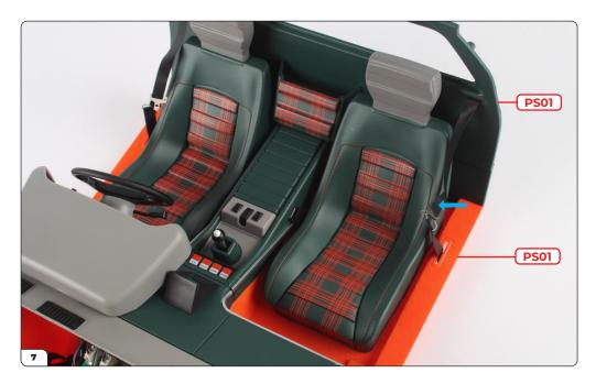
Repeat these steps on the other side to fit the second seat belt, securing with 2x PS01 screws in the same way.
