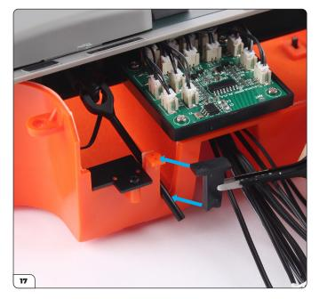
Place the steering column bracket in position.
