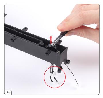
Carefully pull the other wires (from Stage 032) out from the opening.
