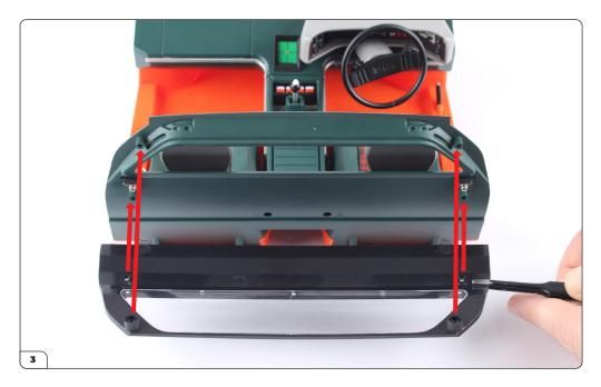
Align the bulkhead glass frame with the bulkhead (stage 049).
