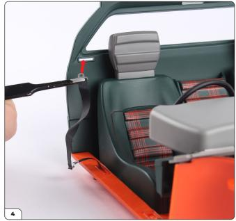
Fit the long end of the seat belt through the opening in the bulkhead.
