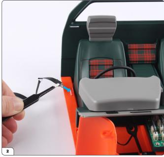
Push the short end of the seat belt through the opening in the cockpit floor. Check that the buckle on the seat belt will face inwards once the upper section of the seat belt has been attached (see image step 6).
