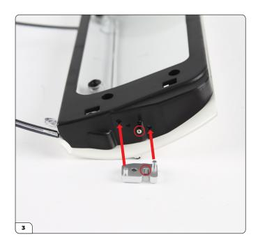
Position the left door lock (54-B) in place, pressing its pins into the holes. At the same time, fit the U-shaped opening under the protruding pin (circled).
