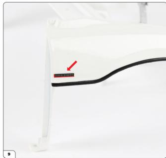
Remove the backing from the front fender plate (inset) then carefully stick it to the front body using the guideline to position it correctly. Make sure the writing is the correct way up.
