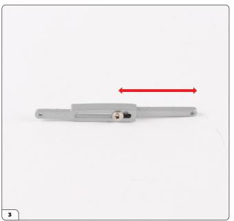
Make sure the screw isn't overtightened, the inner support strut should be able to move back and forth.
