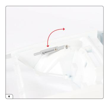
Check that the bonnet support strut can move up and down. Adjust the tightness of the screw if needed.
