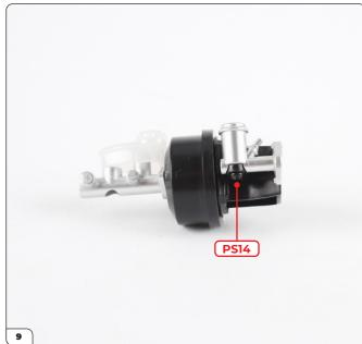
Position the clutch master cylinder (56-C) on the brake servo mounting bracket.
