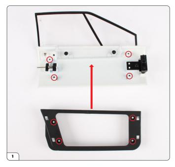
Take the door assembly from Stage 052 and align the left door interior frame (54-A) with it. Position the screw holes over the posts (circled).
