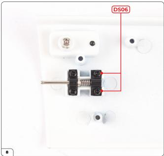
Position the bracket (51-D), compressing the spring against it at the same time. There is a recess on the bracket that fits over the ridge of the door as indicated by the dashed lines.
