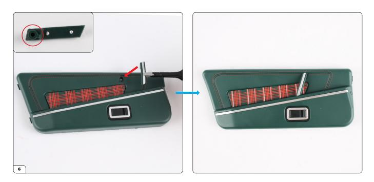
Fit the left pull handle (53-E) using the shaped plug (circled) as a guide.
