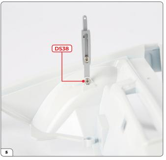
Secure the bonnet support strut by driving through a DS38 screw from the inside as shown.
