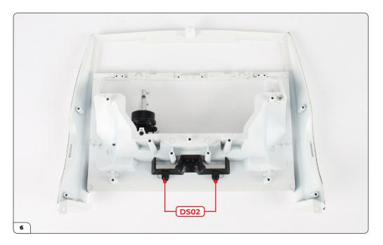
Position the dual air intake and secure it using 2x DS02 screws.
