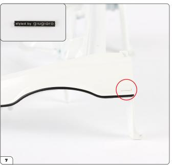
Next take one of the front fender plates (55-D), which have "styled by giugiaro" written on them (inset). Locate the guideline marked on the left-hand side of the front body (circled).
