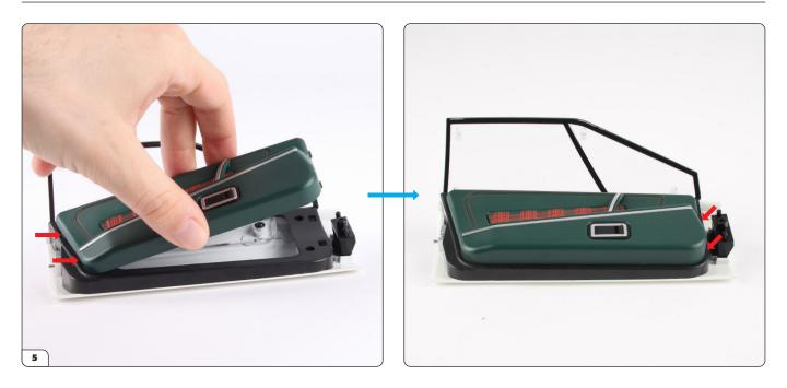
Attach the interior panel (stage 053) to the frame by fitting the tabs into the slots then pressing firmly on the opposite end until it clicks in place.
