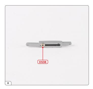
Secure the parts together using a DS38 screw, going through the outer support strut and into the inner one.
