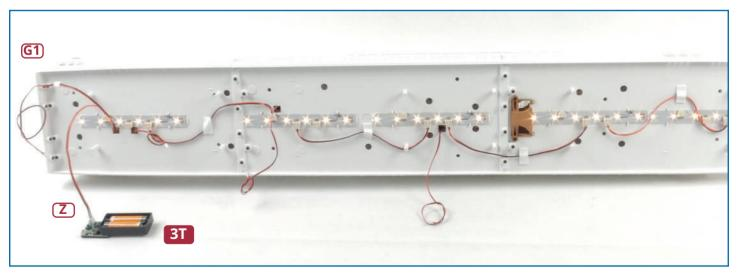
6 When the decks are fixed together, check that the lights are operating correctly by plugging the cables with the G1 and Z connectors, one at a time, in to the tester supplied with issue 3.
