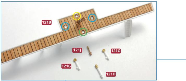
3 Similarly, use a little glue to fix the two telegraphs 121G (shaped holes, circled in blue), the telephone 121H (hole circled in yellow), and the compass 121J (hole circled in green).
