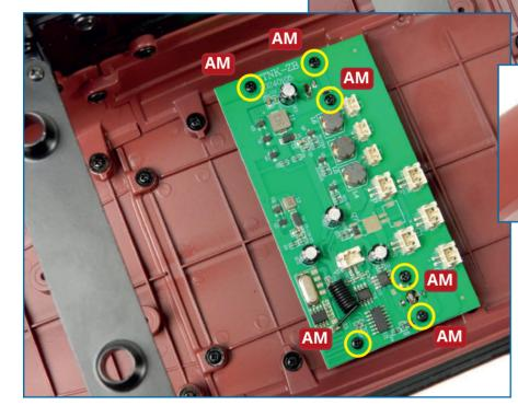
**2** Fit the circuit board **117A** inside the hull so that the power connectors fit in the holes in the hull and the six screw holes in the board are aligned with the screw sockets in the hull. Fix in place using six **AM** screws.
