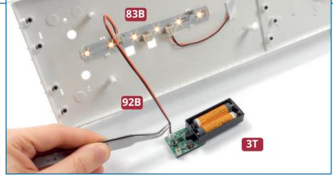
**9** Take the bridge deck and apply four adhesive strips **121D**, as shown above in green, to hold the cables in place. Connect the cable **92B** from the LED strip **83B** to the tester **3T** supplied with issue 3 and check that the lights work. Disconnect the tester after use.
