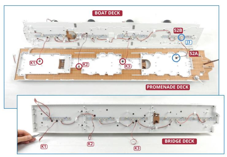
Position the boat deck next to the promenade/bridge deck assembly and pass the ends of cables **K1**, **K2** and **K3** through the holes circled in red. Connect the cable **52A** from
