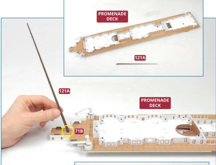
**5** Take the promenade deck and the aft mast **121A**. Fit the end of the mast to section **71B** of the deck and fix it in place from underneath using an **IM** screw.
