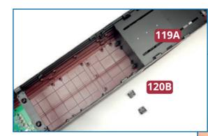
Take the hull of your model and the two brackets **120B**. Identify the fixing points for the brackets near the engine room deckhead **119A**. Fix the brackets in place with four **AM** screws, as indicated.
