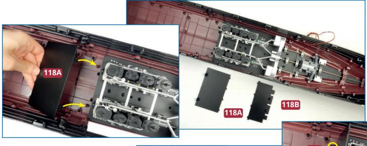
Take the bulkheads **118A** and **118B** and the hull assembly from the previous issue. Position the forward bulkhead **118A** at the end of the reciprocating engines, as indicated, so that the screw holes in the tabs align with the screw holes in the base of the hull. Fix in place with two **NP** screws.
