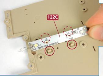
8 Take the LED strip **122C** and connect it to the tester supplied with issue 3, to check that the LEDs are working. Identify the fixing points for part **122C** and fit it in place, inserting one side below the tabs and then clipping the other side in place.
