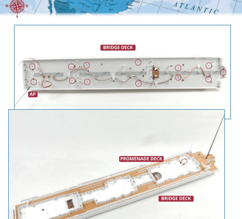
2 When you are happy with the fit of the promenade deck and the bridge deck, identify the thirteen screw holes on the underside of the bridge deck, circled in red (top). Check that the cables are clear of the
