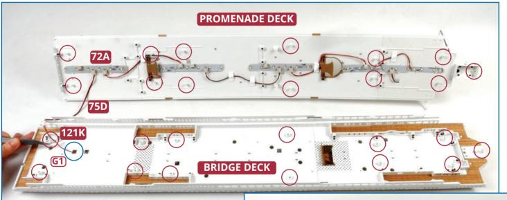
1 Identify the LED strip 72A on the underside of the promenade deck, and the cable that was adjusted in the previous issue, made up of 75D and 121K. Run the G1 end of the cable 121K through the hole in the bridge deck (circled in blue). Fit the promenade deck to the bridge deck: check that all the pegs (circled in red, top) fit into corresponding holes in the bridge deck.
