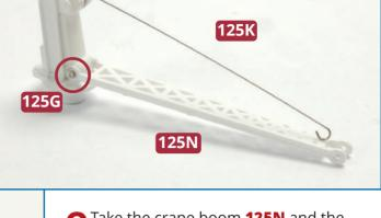
Take the crane boom 125N and the long pin 125G. Fit the eyelets on the wide end of part 125N on either side of the cylindrical structure at the base of part 125B. Fit the pin 125G through the structure, fitting the smooth end first. The crimped end will hold the pin in place. Use a pair of small pliers to squeeze the pin in place.
