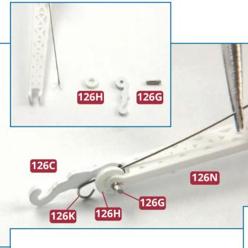
3 Fit the eyelet on the hook 126C and the washer 126H between the eyelets at the narrow end of the boom 126N so that all the holes are aligned. Fit the smaller loop on the cable 126K between the hook and the washer. Fix the hook, cable and washer in place with the short pin 126G. Fit the smooth end first and squeeze the pin in place with pliers.
