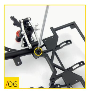
59/06 Turn the chassis upside down and screw a second type B screw into the indicated hole on the underside.
