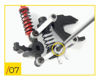
58/07 Finally, position the fork bracket so that it lines up with the arm's central hole, then secure the pieces together using a type C screw.
