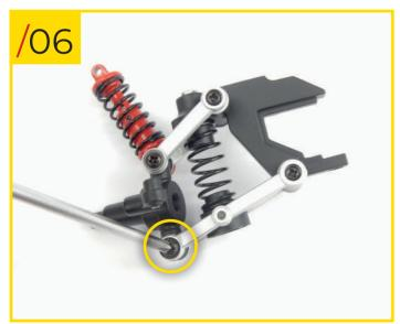
58/06 Screw a type J screw into the hole indicated to secure the arm to the stub axle.
