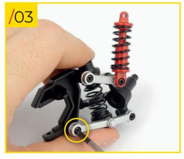
58/03 Connect the lower arm B (the one without a central hole) to the rest of the assembly, orienting the pieces as shown. Line up the longer end of the arm with the mount, and the shorter end with the stub axle, then insert the stud on the centre of the arm into one of the holes in the spring support. Screw a type B screw into the hole indicated by a circle in the photo.
