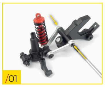
58/01 Place the front right suspension assembly you worked on in stage 57 and the connecting mount on your work surface. Orientate the pieces as shown and secure them together by screwing two type B screws into the holes indicated.
