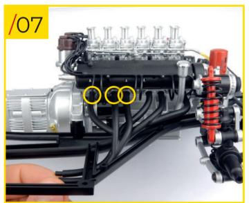
61/08 Insert the stud on the end of the rear exhaust manifolds into the corresponding hole in the chassis, as shown.
