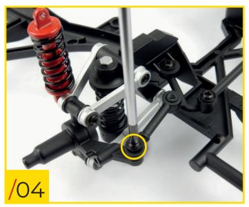
60/04 Connect the front right suspension's stub axle to the right arm using one of the tie rods supplied with stage 59. Orientate the tie rod as shown and secure it to the stub axle using a type J screw (supplied with stage 59).
