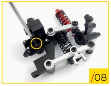
59/09 Fit the steering box insert to the steering box.
