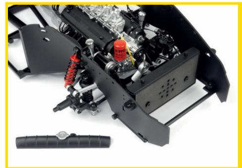
STAGE 64 IS COMPLETE Here's how the first set of radiator components look once they've been correctly fitted. Keep the radiator header in a safe place, you'll need it for a later stage.
