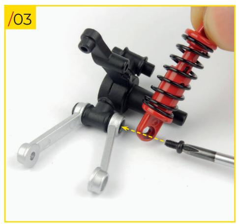
57/03 Now fit the shock absorber to the rest of the assembly, orientating the pieces as shown. Secure everything together using a type C screw.
