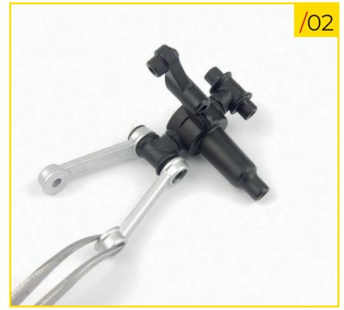
57/02 Fit the second upper arm to the stub axle, being very careful to ensure you orientate the pieces as shown in the photo.
