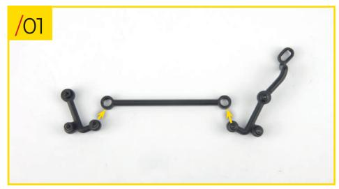
59/01 Place the centre link, idler arm and pitman arm on your work surface, orientating them as shown. Fit the pieces together by inserting the studs on the arms into the respective holes in the centre link.
