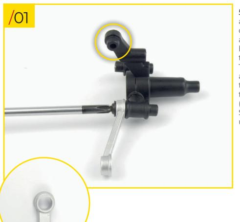
57/01 Fit one of the upper arms to the stub axle, orientating the pieces as shown. Use the stud highlighted by the circle in the photo as a reference. The holes at the ends of the arms aren't identical: for this step you'll need to use the end with the larger hole (shown in the round photo). Secure the pieces together using a type J screw.
