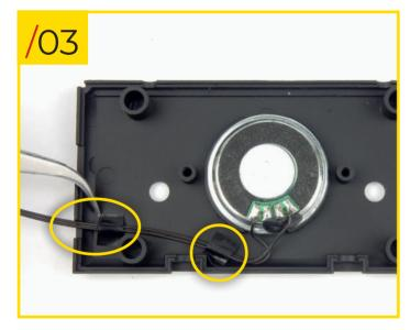
64/03 Position the speaker cable as shown, to ensure it exits from the side of the housing panel. To avoid damaging the cable during the assembly process, we recommend taping it to the panel as indicated in the photo.
