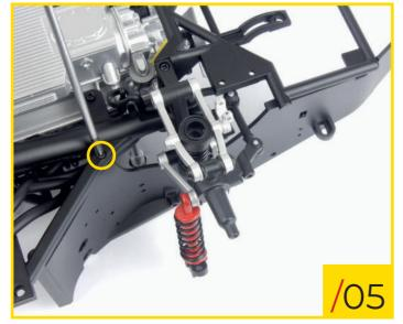
62/05 Turn the assembly over and finish securing by screwing a third type B screw into the hole indicated.
