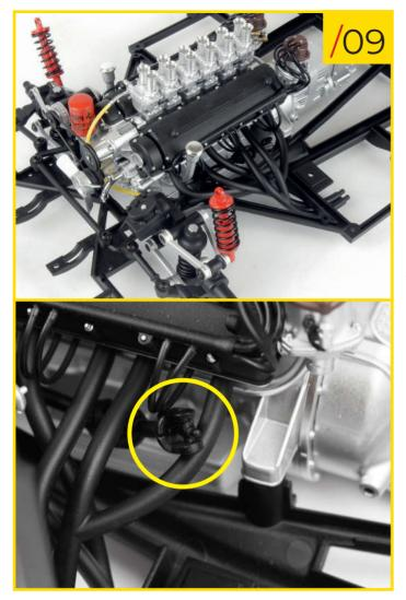
61/09 Repeat the previous steps to fit the left-side exhaust manifolds.
