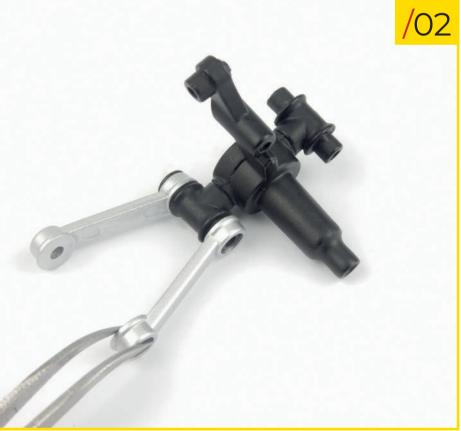
57/02 Fit the second upper arm to the stub axle, being very careful to ensure you orientate the pieces as shown in the photo.
