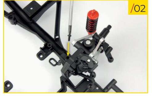
60/02 Screw a type B screw (supplied with stage 59) into the hole indicated in the photo.
