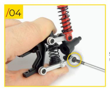
58/04 Secure the arm to the stub axle using a type J screw.
