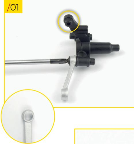
57/01 Fit one of the upper arms to the stub axle, orientating the pieces as shown. Use the stud highlighted by the circle in the photo as a reference. The holes at the ends of the arms aren't identical: for this step you'll need to use the end with the larger hole (shown in the round photo). Secure the pieces together using a type J screw.
