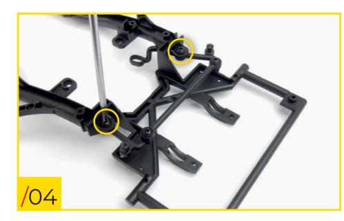
59/04 Secure the arms to the chassis by screwing two type J screws into the holes indicated in the photo.
