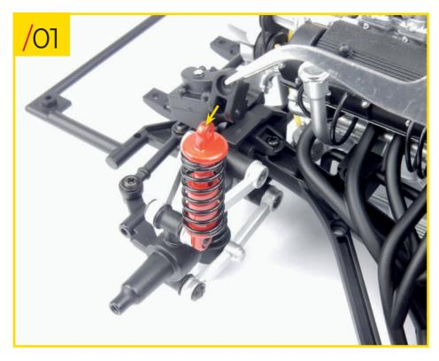
62/01 Fit the bracket to the front left shock absorber. Orientate the pieces as shown in the photo.
