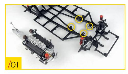
61/01 Place your model's engine and chassis on your work surface. Look at the photo carefully to identify the holes and mounts (indicated by the circles) that you'll need for fitting the engine.
