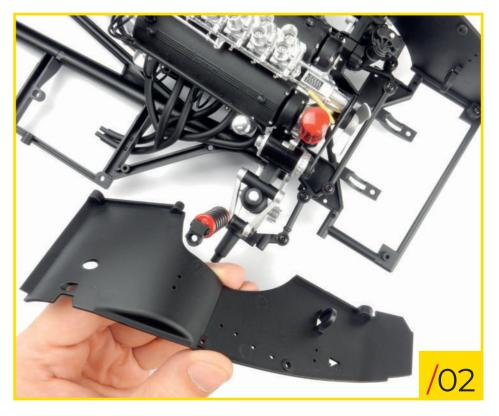
63/02 Fit the front right inner wing to the chassis, orientating the pieces as shown.
