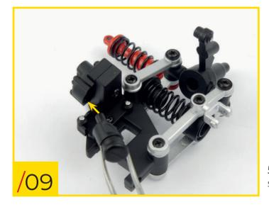
59/07 Fit the steering box to its mount, orientating the components as shown. Secure the pieces together using a type B screw.
