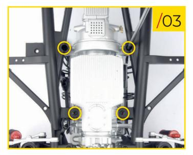
61/03 Turn the assembly over and secure the pieces together using four type C screws.
