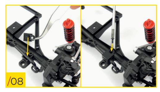
60/08 Fit the mounting plate to the chassis and secure it in place using a type B screw.
