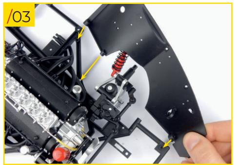
62/03 Fit the front left inner wing to the chassis, orientating the pieces as shown.
