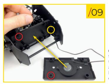
64/09 Thread the speaker cable through the opening indicated by the yellow circle in the photo. Press the speaker housing panel and back panel together, using the holes highlighted by the red circles in the photo to orientate the components correctly.
