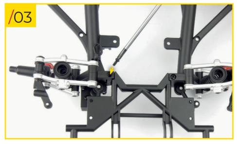
60/03 Turn the chassis upside down and screw a second type B screw (supplied with stage 59) into the hole indicated in the photo. Tighten the screw to ensure the suspension is securely fitted to the chassis.
