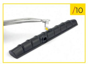
64/10 Fit the radiator cap to the radiator header by orientating the pieces as shown and inserting the stud on the cap into the hole in the header.
