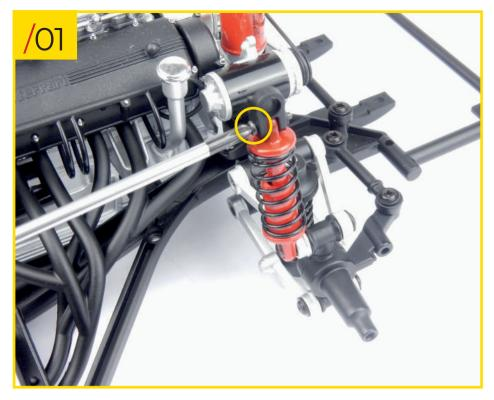
63/01 Fit the bracket to the front right shock absorber. Orientate the pieces as shown in the photo and secure them together using a type G screw.
