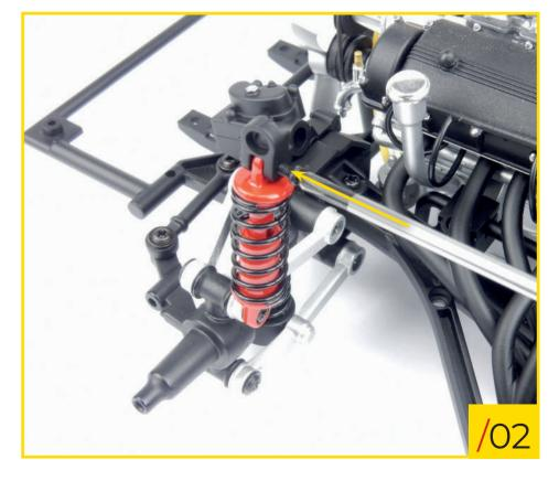
62/02 Secure the bracket to the shock absorber using a type G screw.
