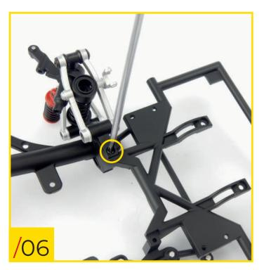
59/06 Turn the chassis upside down and screw a second type B screw into the indicated hole on the underside.
