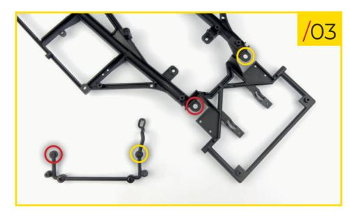
59/03 Retrieve your model's chassis, orientate it as shown and fit the steering assembly to it. The circles in the photo show which studs on the arms need to go into which holes in the chassis.
