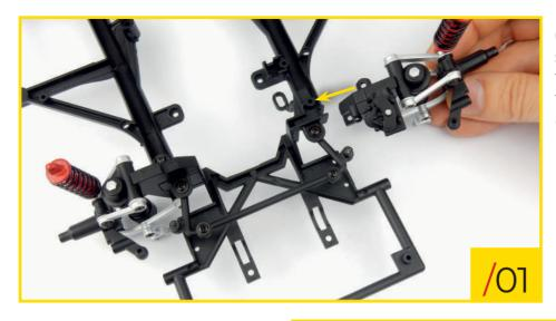
60/01 Retrieve the front left suspension and chassis from stage 59. Fit the pieces together, orientating them as shown.
