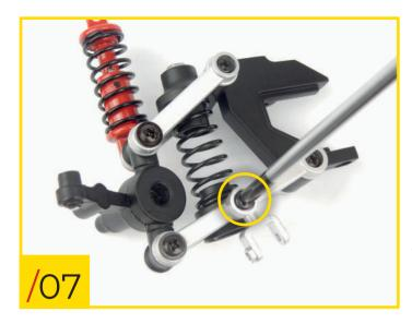
58/07 Finally, position the fork bracket so that it lines up with the arm's central hole, then secure the pieces together using a type C screw.
