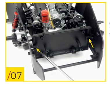
64/08 Turn the assembly over and, working on the underside of the chassis, screw another two type B screws into the holes indicated by the arrows in the photo. 64/07 Screw two type B screws into the holes indicated to secure the panel to the chassis.
