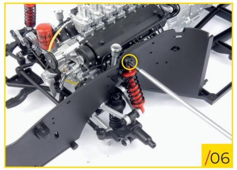
62/06 Secure the left shock absorber bracket to the inner wing with another type B screw.
