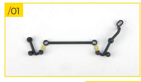
59/01 Place the centre link, idler arm and pitman arm on your work surface, orientating them as shown. Fit the pieces together by inserting the studs on the arms into the respective holes in the centre link.
