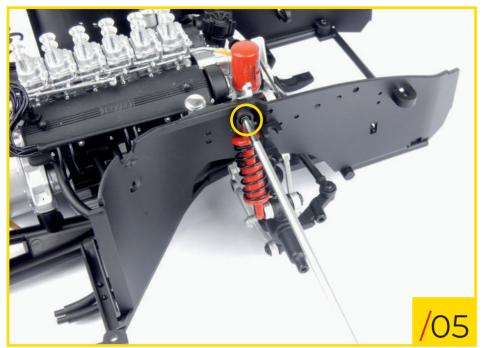
63/05 Secure the right shock absorber bracket to the inner wing with another type B screw.
