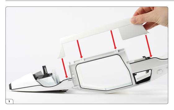
Carefully place the main body (stage 068) upside down, using a soft surface to protect the paintwork. Align the right rocker panel (69-A) with the main body.
