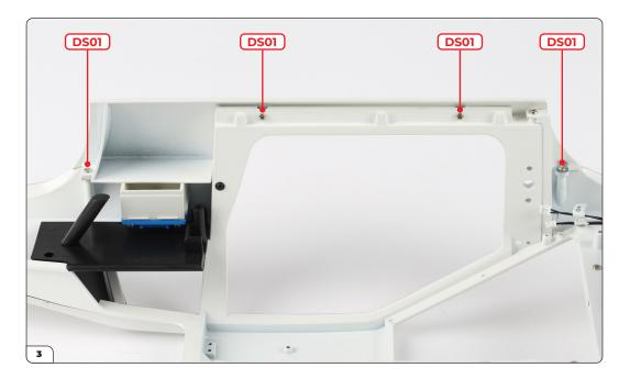
Screw the rocker panel to the main body with 4x DS01 screws.
