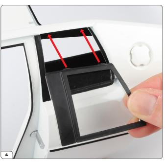
Take the main body and open the left door. Align the two tabs on the top of the frame with the main body.
