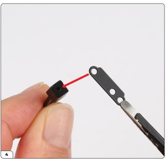
Align the other tailgate hinge (75-C) with the right tailgate bracket (75-A) as shown.
