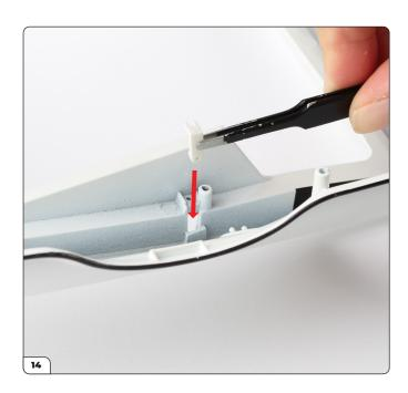
Push the left bracket (68-F) into the main body on the rear left side.
