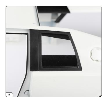
Push the tabs in place then press the quarter frame into the main body.
