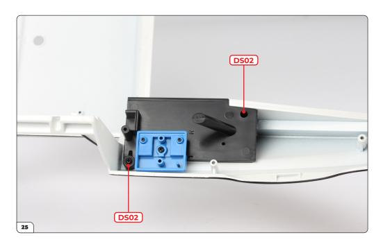
Screw the right chassis plate to the main body using 2x DS02 screws.
