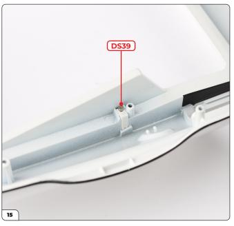
Screw the bracket in place with a DS39 screw.
