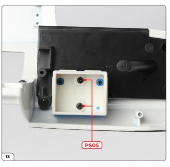
Press the battery onto the battery cover. Screw the parts together with 2x PS05 screws.
