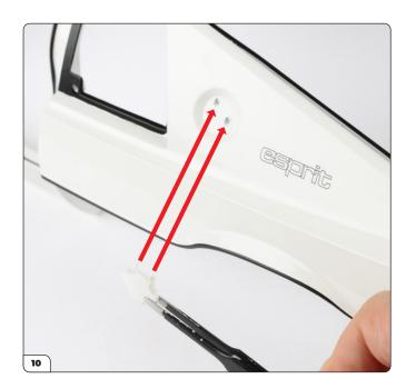
Align the left fuel cap (68-E) with the main body (stage 067).
