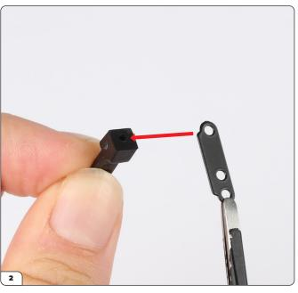
Align a tailgate hinge (75-C) with the left tailgate bracket (75-B) as shown.
