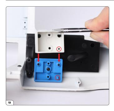
Align the battery (68-B) with the battery cover (stage 067). There is a pin (circled) to ensure the parts are fitted together correctly.
