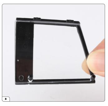
Press the window onto the frame.
