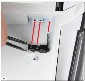
Align the right tailgate bracket (marked "R") and hinge with the main body.
