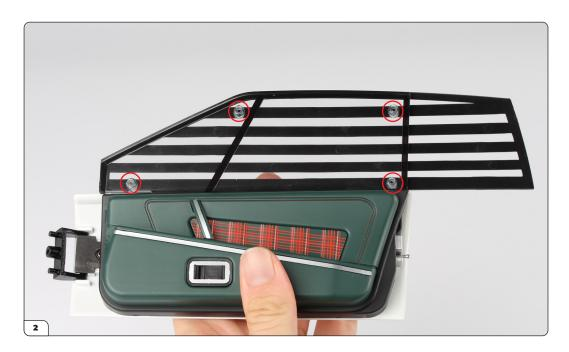
Push the window louvres onto the right door window. Check that the screw posts (circled) are firmly in place.
