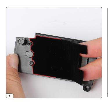
Stick the sticker to the chassis plate, starting with the edge highlighted by the red line.
