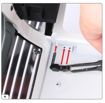
Carefully place the main body (stage 074) upside down. Align the left tailgate bracket (marked "L") and hinge with the main body.
