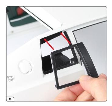
Open the right door. Align the two tabs on the top of the frame with the main body.
