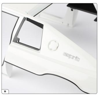
Press the fuel cap firmly in place.
