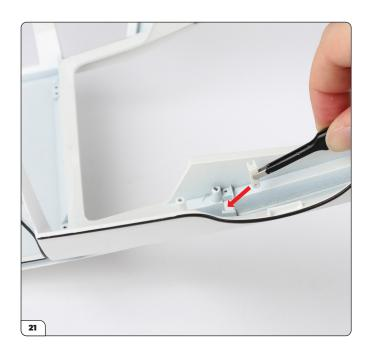
Push the right bracket (67-F) into the main body on the rear right side.
