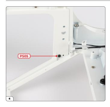
Screw the right panel to the main body with a PS05 screw.
