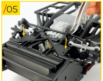
66/05 Insert the studs on the brackets into the respective holes in the chassis, as shown in the photo.
