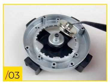
69/03 Place the type B hub onto the jig's central stud; once in place, put the type A hub on top of it, as shown in the photo.
