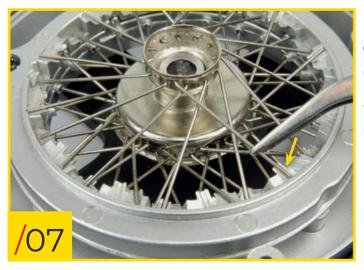
71/07 Place the straight end of the spoke onto the corresponding notch on the top level of the housing. Repeat these steps for the other eleven type C spokes, until all the holes in the top row on the hub have been filled.
