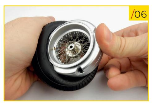
72/06 Slip the tyre onto the rim of the rear left wheel.
