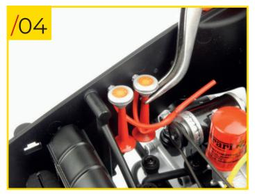
67/04 Retrieve your model's chassis and install the two horn assemblies to the internal face of the front right inner wing.
