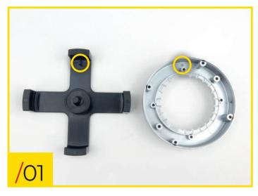
69/01 Place the assembly jig you received in stage 21 on your work surface, together with the wheel rim supplied with this stage. The jig has a small fixing stud on it, this should be inserted into the corresponding hole in the rim.
