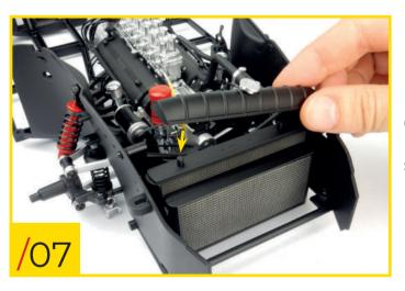
65/07 Carefully press the header onto the rest of the radiator. Orientate the pieces as shown in the photo.
