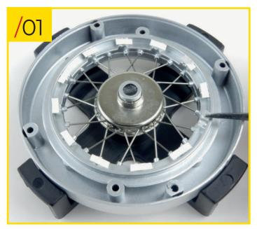
70/01 Place the rear left wheel that you assembled in stage 69 on your work surface. Before proceeding, we recommend that you stick small strips of double-sided sticky tape to the side edge of the spoke retainer ring 1. Alternatively, you can lay all the spokes in position and then dab a bead of glue on each one after stage 70/03.
