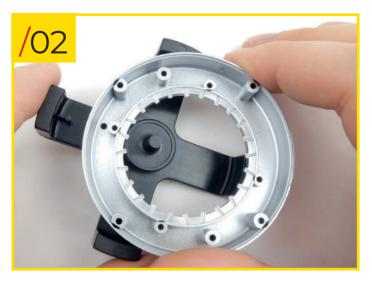
69/02 Insert the stud into the hole to fix the rim onto the assembly jig. Before proceeding with the assembly, we recommend that you stick a small piece of double-sided sticky tape to the jig's central stud - this will help to hold the hubs in place.
