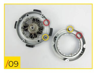
71/09 Fit the outer wheel rim to the rest of the wheel. To line up the fixing holes, match up the arrows circled in red.
