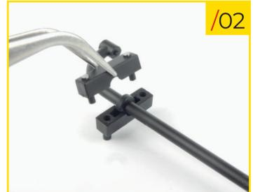
66/03 Fit the two halves of the other bracket onto the ring at the other end of the anti-roll bar.
