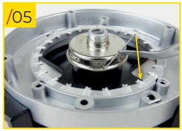
69/05 Position the type B spokes (they are shorter than the type A ones) by inserting their hooked end into the lower row of holes in the type A hub. Place the straight end of the spokes onto the corresponding notch on the edge of the rim (on the double-sided sticky tape). Always leave an empty hole between each spoke.
