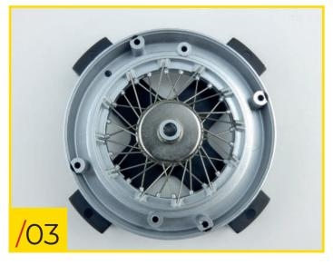
70/03 Look at the photo to check that you've correctly installed the type A spokes.
