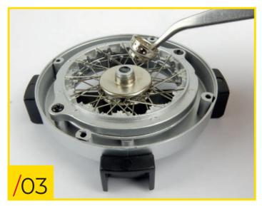
71/04 Insert the hooked end of one type C spoke into one of the holes in the lower row on the type C hub.
