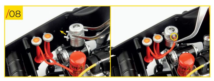
67/08 Fit the compressor to the internal face of the front right splash guard, close to the horns, and slide the free end of the short tube onto the stud on the compressor cover.
