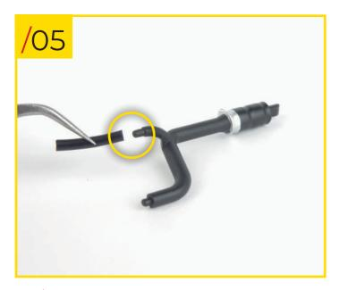
65/05 Slide the flexible hose onto the stud on the short end of the radiator hose.
