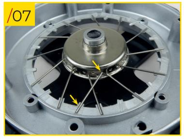
69/07 Now position the type A spokes (they are longer than the type B ones) by inserting their hooked end into the upper row of holes immediately to the left of the type B spokes, making sure they pass over the spokes inserted into the lower row of holes. Use the photo to help identify which notch you should position the other end of the spoke on. Leave an empty hole between each spoke as before.
