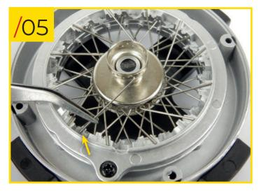
71/05 Place the straight end of the spoke on the notch on the lower level of the retainer ring as shown in the photo. Repeat these steps for the other eleven type C spokes, until all the holes in the lower row on the hub have been filled.
