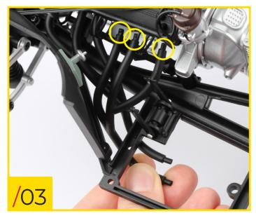
/03 Pull the three pins (circled) out from the engine.
