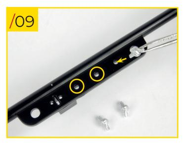
80/09 Insert the semi-circular ends of the three C switches into the dedicated semi-circular holes in the central section of the dashboard support. There's only one way that the pieces can be secured together.
