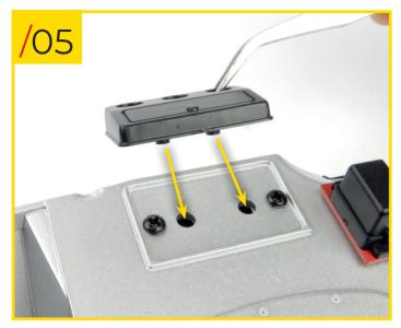
80/05 Fit the pipe housing to the firewall, into the position shown in the photo. Insert the studs on the housing into the dedicated holes in the firewall.
