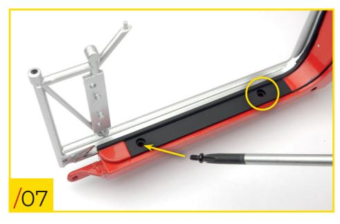
75/07 Screw two type C screws into the holes indicated to secure the footboard to the body.
