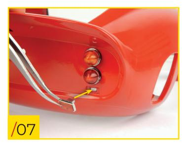
73/07 Finally, fit the second reflector to the right side of the body.
