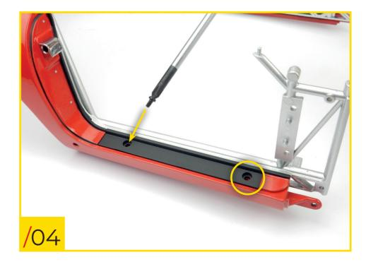
76/04 Screw two type C screws into the holes indicated to secure the footboard to the body.
