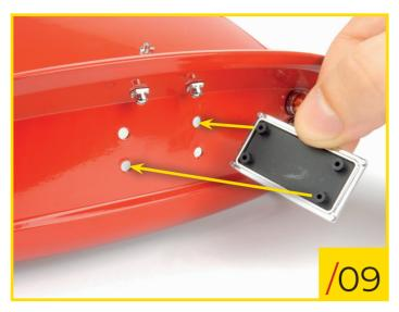
74/09 Fit the number plate assembly to the rear section of the body by inserting the studs into the dedicated holes.
