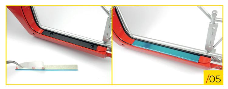
76/05 Remove the protective film from the back of the plate and place it in the orientation shown onto the black part of the footboard to hide the screws. Don't remove the blue film yet, it will protect the surface of the plate during future assembly sessions.
