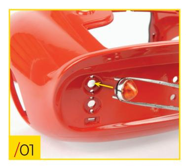
73/01 Place the rear section of the body (stage 68) on your work surface. Fit one of the indicators into its position on the left side of the body, orientating the parts as shown.
