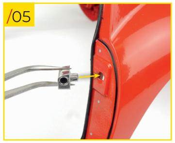
74/05 Put the left door lock into its hole in the rear section of the body. Orientate the pieces as shown: the hole in the lock should be facing outwards.
