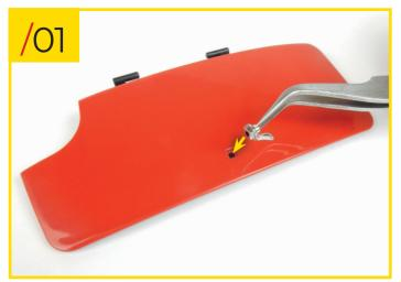
74/01 Add the boot lock to the boot lid, orientating the pieces as shown. Before placing the lock into position, we recommend that you use a type L screw to enlarge the hole, this will make the next step easier to complete.
