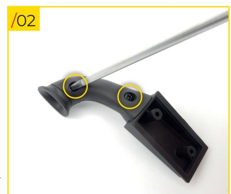
77/02 Secure the pieces together using two type M screws.
