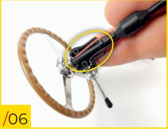
79/06 Retrieve the steering wheel assembly that you assembled in stage 1, and fit steering base A to it. Orientate the pieces as shown and be careful not to damage any of the components, particularly the cables. Make sure both cables are threaded through the notch.
