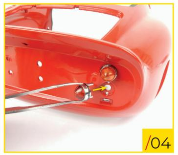
73/04 Press the second brake/parking light into position on the right side of the body, below the indicator.
