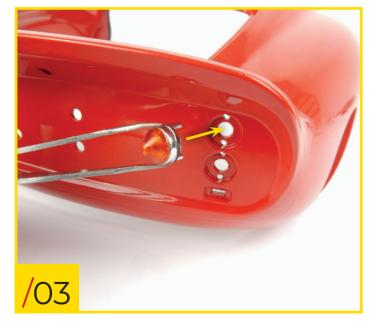
73/03 Fit the second indicator into position on the right side of the body.
