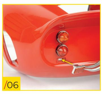
73/06 Place the first reflector into the rectangular hole on the left side of the body, below the indicator and brake/parking light.
