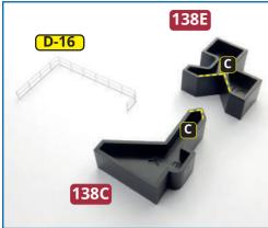
11 Bend part D-16 at right angles, using the two templates 138C and 138E. Then glue part D-16 in place at the port side of the bow skylight, continuing the run of part A-16.
