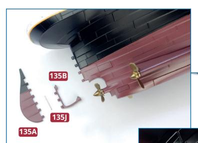
Take the rudder 135A, the hinge 135B and the hinge pin 135J. Check the fit of the hinge at the stern end of the hull and glue in place at the points circled in blue. Fit the rudder so that the loops interlock with the loops on the hinge and at the rear of the stern. Fix in place with the pin 135J, inserting the smooth end first, from the lower end of the rudder.
