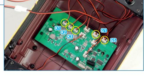
**5** Check that the three smoke generators are working by switching on the batteries (or power pack). The smoke generators, like the motor for the propellers,
