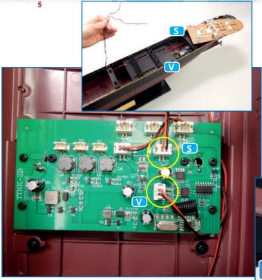
Rest the poop deck and aft well deck on the stern end of the hull, without fixing it. Run the electric cable from the LED board beneath the deck under the crosspieces and connect it to the socket marked S on the circuit board. Do the same with the cable from the motor and connect it to the socket marked V.
