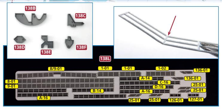
**5** The photo-etched parts are the railings for various parts of the ship. The plastic templates are provided to help you bend them accurately. Each angle on the template has a letter, and the letters have to be matched together to provide both sides of the shape to be formed.
