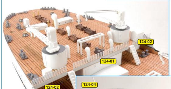
Remove parts 124-01, 124-02 (x2), 124-03 (x2), 124-04, 125-02 (x4), 133-01 and 134-01 from plate 140K. Bend the parts using the curves M on templates 139A and 138B, and angles B on templates 138E and 138F. Glue the parts in place on the poop deck and cranes as shown in the photos below. The railings 125-02 are fitted on either side of the steps down to the aft well deck.
