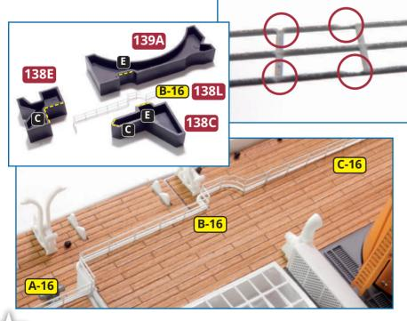
Take the photo-etched parts 138L (from issue 138) and remove part B-16 from the frame. Bend it with shapes C and E on templates 138C, 138E and 139A. Note the notches on the part, indicating where the part should be bent (circled, above) Match the letters on the templates to bend the railing correctly. Glue part B-16 between parts A-16 and C-16, on the starboard side of the model.
