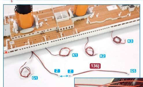
Join the connector marked Z on the cable 136J to the cable marked Z coming from the underside of the deck assembly. Connect the cables marked K1, K2 and K3 (from the funnels) and G1 and G5 to the corresponding sockets on the main circuit board.
