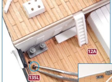
9 Fit four more screw eyes 135L at the corners of the well deck 12A at the points circled in blue.
