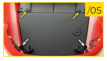
89/05 Retrieve the boot frame that you worked on in stage 75 and fit it into its position. Secure it in position with two type B screws (yellow arrows) and two type C screws (white arrows).
