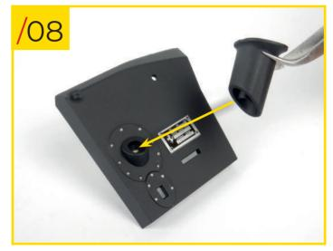
82/08 Fit the air duct into its dedicated position on the panel.
