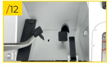
88/12 Fit the clutch pedal into its position on the front of the firewall. There's only one way that the pieces can fit together.
