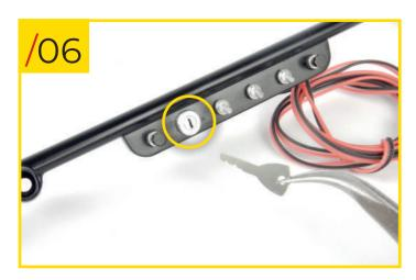
81/06 Fit the ignition switch to the front of the support and insert the key into the hole. The components are very fragile, be careful not to damage them.
