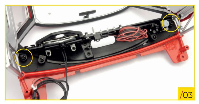
84/03 Also retrieve the dashboard support and install it as shown in the photo. Secure the pieces together using another two type C screws (stage 81).
