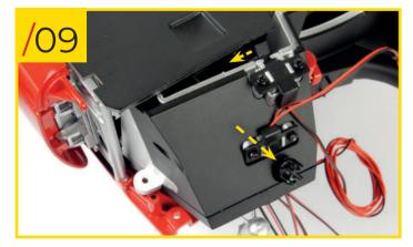
89/09 Retrieve the firewall and fit it to the rest of the model, making sure the steering column goes through the dedicated hole.
