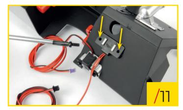
88/11 As before, use two type B screws to secure the brake pedal assembly to the rear of the firewall.
