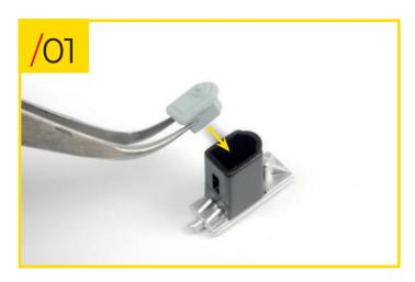
81/01 Fit the cover to the windscreen wiper motor by pressing it into place.
