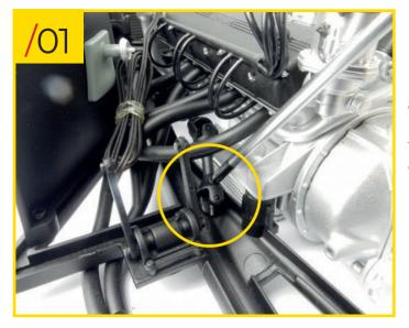
82/01 Retrieve the chassis assembly and remove the screw, the tab at the end of the axle, and the cross-shaped central component from the steering shaft.
