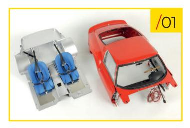
89/01 Place the rear section of the body and the body floor on your work surface.
