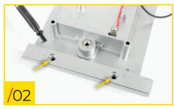
90/02 Fit the left plate (marked with the letter "L") into its position and secure it in place with two type B screws.
