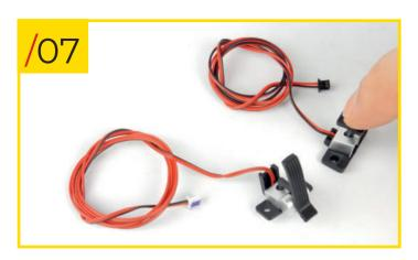
88/07 Press the two pedals you've assembled so far to check that their switches are working properly.
