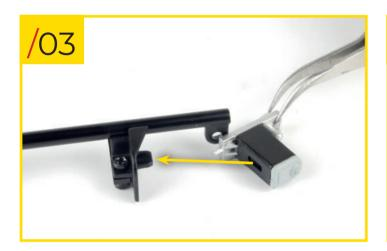
81/03 Fit the windscreen wiper motor to the bracket. Orientate the pieces as shown.
