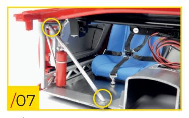
89/07 Fit the support rod into the position indicated in the photo, on the right side of the passenger compartment. Orientate the pieces as shown.
