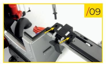
88/09 Screw two type B screws into the holes indicated to secure the accelerator pedal assembly to the rear of the firewall.
