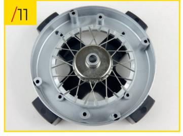
84/11 Now position the type A spokes (they are longer than the type B ones) by inserting their hooked end into the upper row of holes immediately to the left of the type B spokes, making sure they pass over the spokes inserted into the lower row of holes. Always leave an empty hole between each spoke as before.
