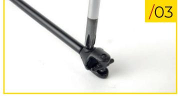
82/03 Use the screw that you removed in step 01 to fit the tab and central component to the end of the steering column. Look at the photo to check that you've fitted the pieces together correctly.
