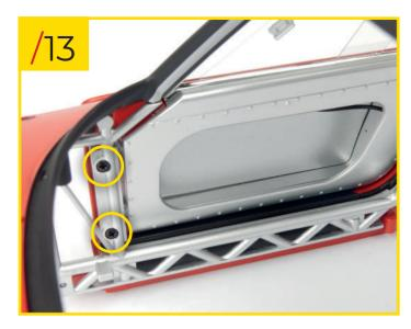
83/13 Screw two type C screws (from stages 75 and 76) into the holes indicated. Repeat steps 12 and 13 to fit the left door to the body as well.
