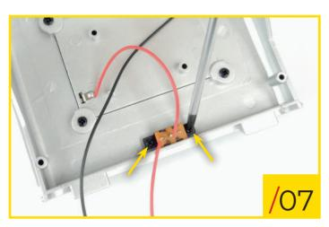
90/07 Secure the switch to the battery tray base using two type L screws.
