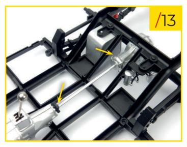
90/13 Finally, retrieve the prop shaft with the coupling that you assembled in stage 88 and fit it to the position indicated on the chassis to connect the gearbox to the differential.
