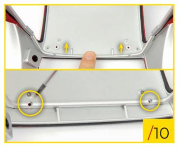
83/10 Push the roll-bar inwards until its holes line up with the raised holes on the roof. Push upwards to insert the sub-frame studs completely and then screw two type N screws (step 75) into the holes indicated.
