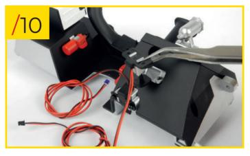
88/10 Now fit the brake pedal assembly into its position. Use the photo to help orientate the components correctly.
