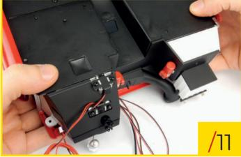
89/11 Make sure the profile of the firewall lines up with that of the body floor.
