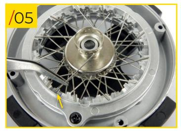
86/05 Use the photo to help put the straight end of the spoke on the notch on the lower level of the retainer ring. Repeat these steps for the other eleven type C spokes, until all the holes in the lower row on the hub have been filled.
