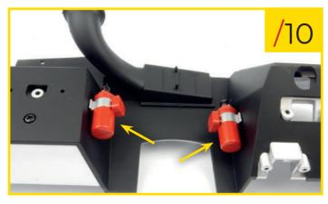
81/10 Retrieve your model's firewall assembly and fit the two coils to its inner side. Some light pressure will need to be applied to fit the pieces together.
