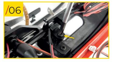
84/06 Retrieve the switch bracket that you assembled in stage 81 and install it into its position on the underside of the dashboard, so that it corresponds with the control positioned between the steering wheel and the key. Secure it into position using a type B screw (stage 81).
