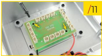
90/11 Fit the printed circuit board to the inside of the battery tray and secure it in place using two type B screws. Orientate the components exactly as shown in the photo.
