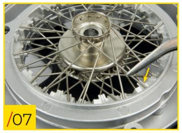
86/07 Place the straight end of the spoke onto the corresponding notch on the top level of the retainer ring. Repeat these steps for the other eleven type C spokes, until all the holes in the top row on the hub have been filled.
