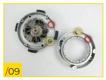
86/09 Fit the outer wheel rim to the rest of the wheel. To line up the fixing holes, look at the photo and match up the circled elements.
