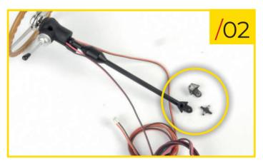
82/02 Retrieve your model's steering assembly and fit the components you removed in step 01 to the end of the steering column.
