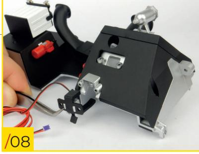
88/08 Retrieve your model's firewall and fit the accelerator pedal assembly into its position. Orientate the pieces as shown.
