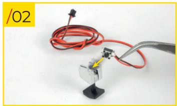
88/02 Fit the brake cable switch (black connector) as shown in the photo. The cable should be facing towards the "tooth" on the pedal.
