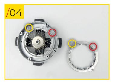
85/04 Add the spoke retainer ring 2 to the rest of the assembly. Use the photo to help fit it correctly.
