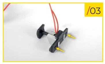
88/03 Fit the brake pedal bracket to the rest of the assembly. Press until the two tabs on the base are fully interlocked.
