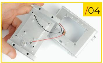
90/04 Insert the battery tray into the hole in the centre of its base. Orientate the pieces as shown in the photo.
