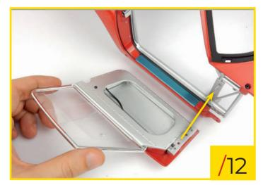
83/12 Retrieve the right door and fit it to the body. Insert the sub-frame studs into the respective holes in the door hinge.
