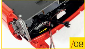
89/08 To make the next steps easier to complete, we recommend that you use some tape or a cable tie to group and tie together the cables coming from the dashboard
