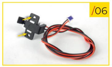
88/06 Fit the accelerator pedal bracket to the rest of the assembly. As before, press until the two tabs on the base are fully interlocked.
