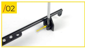
81/02 Retrieve the dashboard support and place the motor bracket into the position indicated in the photo. Secure the pieces together using a type B screw.
