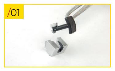
88/01 Fit the brake pedal to its base. Orientate the pieces as shown: the "tooth" on the pedal goes into the corresponding groove in the base.
