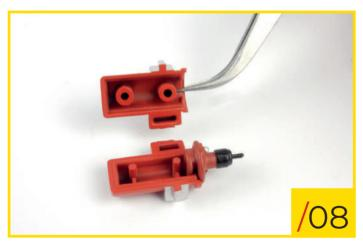
81/08 Fit one of the caps into its position on the inner side of part A of one of the coils and complete the coil by adding part B. Orientate the pieces as shown in the photo.
