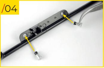
81/04 Working on the rear of the support, insert the two controls into the holes indicated. Do not use glue.
