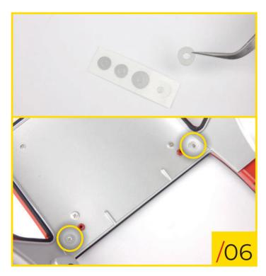
83/06 Detach the two larger stickers from the strip and place them over the heads of the screws used to secure the roof to the body.
