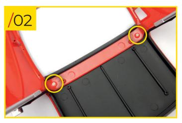
83/02 Working inside the assembly, screw two type N screws into the holes indicated to secure the pieces together.
