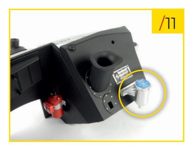
82/11 Fit the brake fluid reservoir to the bracket and add the reservoir cover.
