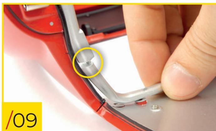
83/09 Introduce the studs on the sub-frame to the holes at the end of the roll-bar, but don't push them all the way in.
