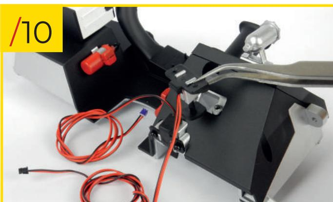
88/10 Now fit the brake pedal assembly into its position. Use the photo to help orientate the components correctly.
