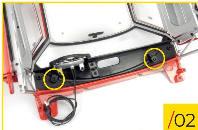
84/02 Retrieve the dashboard and fit it into its position inside the body. Use two type C screws (from stage 81) to secure it in place.
