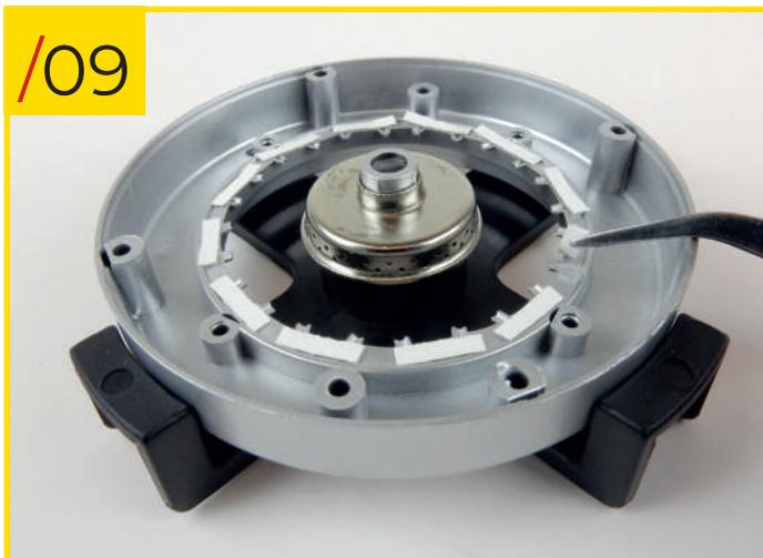
84/09 Place the type B hub onto the jig's central stud; once in place, put the type A hub on top of it. Before adding the spokes, we recommend that you stick some small strips of double-sided sticky tape to the internal edge of the rim, or dab a bead of glue on each spoke once they are in position.
