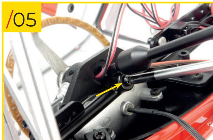
84/05 Working on the underside of the dashboard, screw one type B screw (stage 81) into the hole indicated to secure the pieces together.
