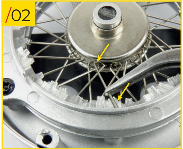
86/02 Insert the hooked end of the type A spokes into the remaining holes in the type A hub. Use the photo to help orientate the spokes correctly and to put their straight end on the corresponding notch on the top level of the housing.
