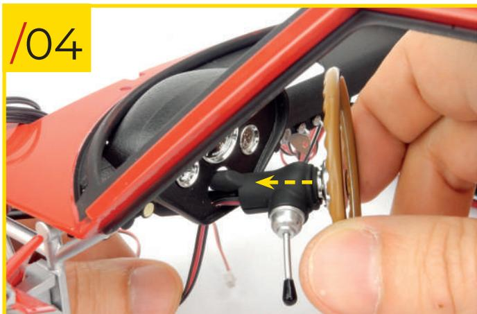
84/04 Retrieve the steering wheel and insert the steering column, with both cables, into the dedicated hole in the dashboard.
