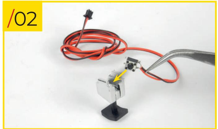
88/02 Fit the brake cable switch (black connector) as shown in the photo. The cable should be facing towards the “tooth” on the pedal.
