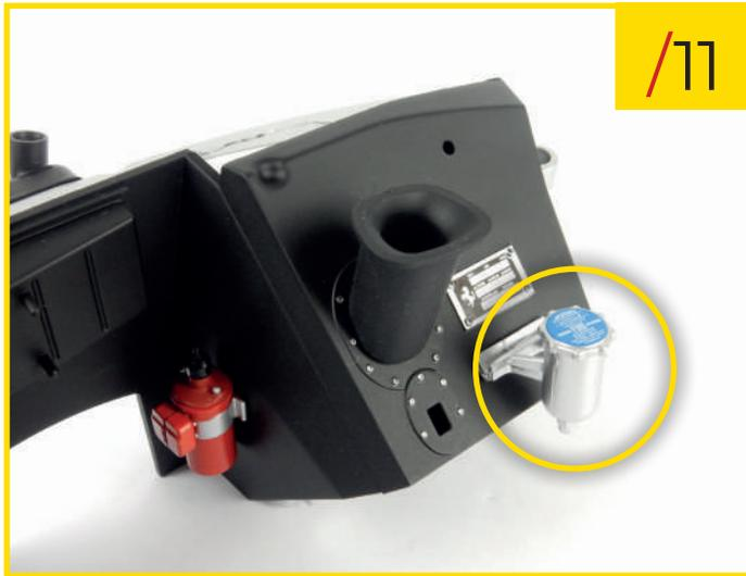
82/11 Fit the brake fluid reservoir to the bracket and add the reservoir cover.
