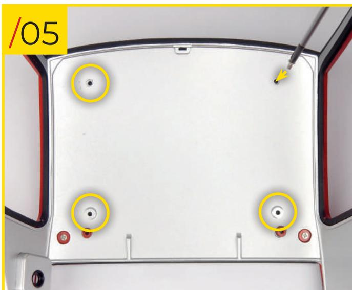
83/05 Fit the head lining to the roof and body, use the shape of the pieces to ensure you orientate them correctly. Screw four type N screws into the holes indicated.
