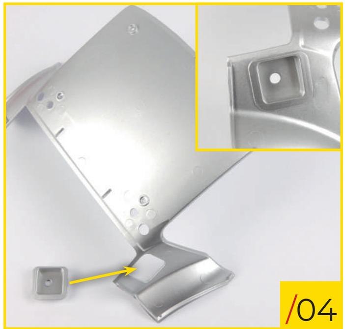
83/04 Insert the fuel tank filler plate into its dedicated position on the head lining.
