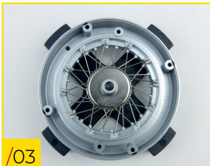
85/03 Look at the photo to check that you've correctly installed the type A spokes.
