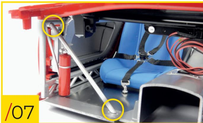
89/07 Fit the support rod into the position indicated in the photo, on the right side of the passenger compartment. Orientate the pieces as shown.
