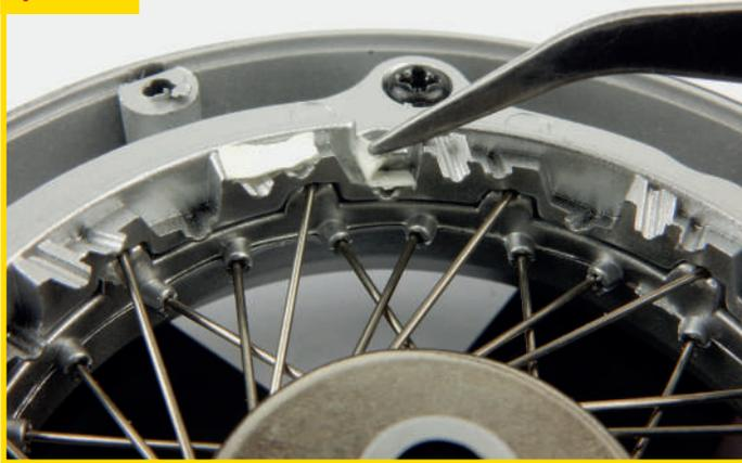
86/01 Place the rear right wheel that you assembled in the previous stages on your work surface. Before proceeding with the assembly, we recommend that you stick small strips of double-sided sticky tape to the side edge of the spoke retainer ring 2. Alternatively, you can add a bead of glue to the spokes once they are in position.
