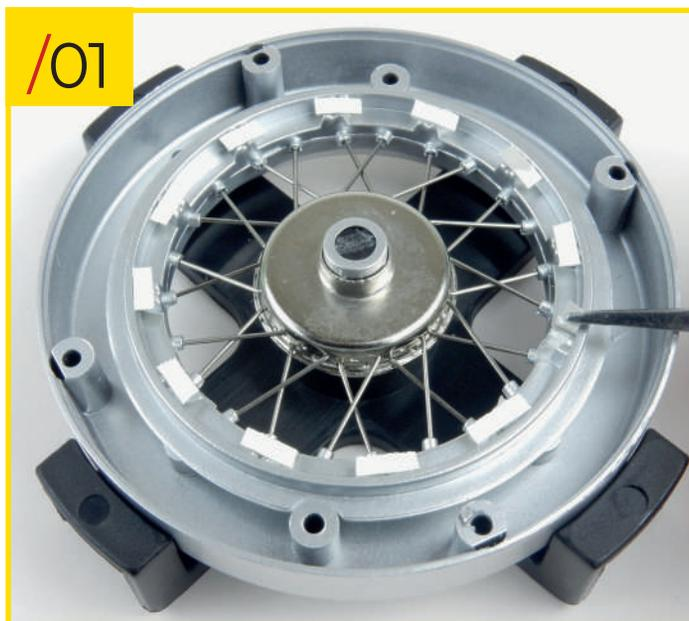
85/01 Place the rear right wheel that you assembled in stage 84 on your work surface. Before proceeding, we recommend that you stick small strips of double-sided sticky tape to the side edge of the spoke retainer ring. Alternatively, you can lay all the spokes in position and then dab a bead of glue on each one after step 85/03.
