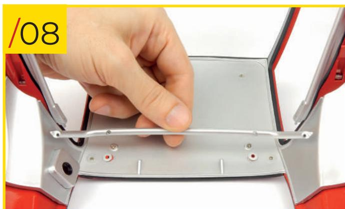
83/08 Retrieve the roll-bar that you received with stage 75 and place it inside the body, orientating it as shown.
