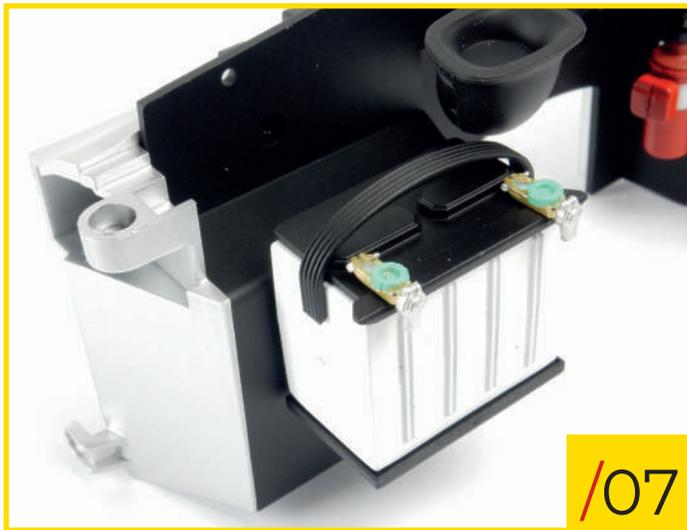
82/07 Add the two battery terminals and the handle to the assembly.
