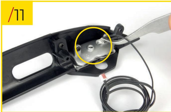
81/11 Retrieve the dashboard assembly and insert the LED light on Cable 1 (red connector) into the hole on the rear of the instrument panel. Be careful not to damage the cable.
