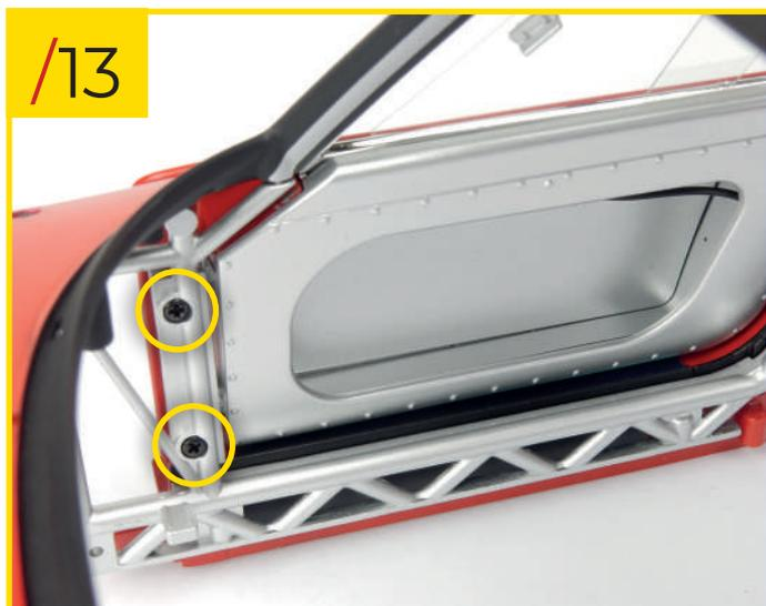
83/13 Screw two type C screws (from stages 75 and 76) into the holes indicated. Repeat steps 12 and 13 to fit the left door to the body as well.
