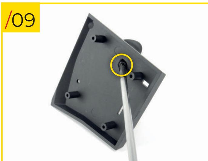
82/09 Working on the underside of the panel, secure the duct to the panel using a type B screw.
