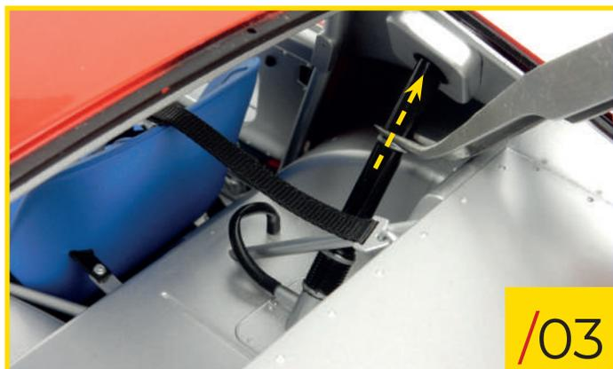
89/03 Push all the components up against each other and insert the end of the oil inlet hose into the hole in the reservoir.
