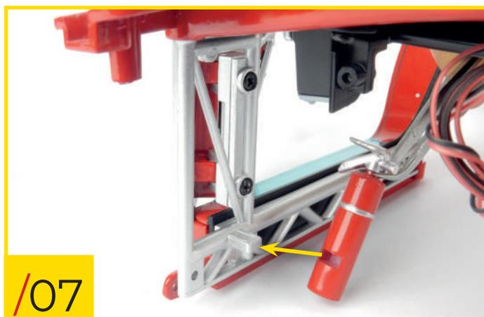
84/07 Retrieve the extinguisher (stage 75) and fit it to the sub-frame of the right door, orientating the pieces as shown.
