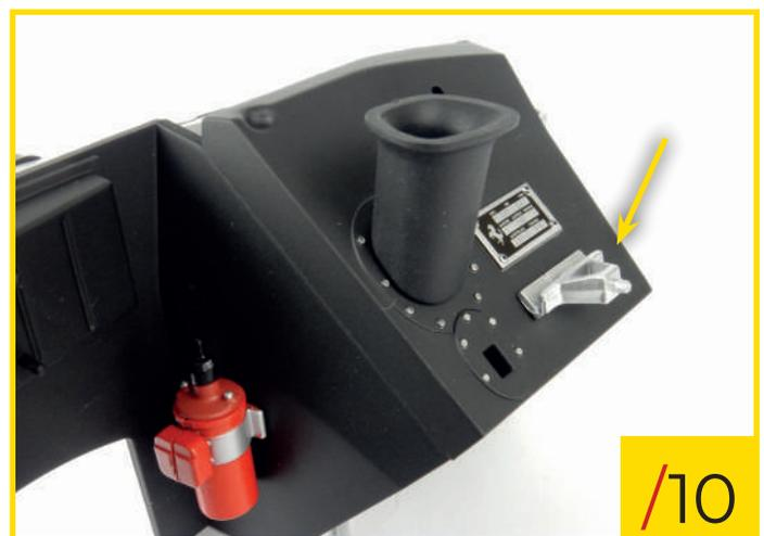
82/10 Use a little pressure to fit the panel to the firewall and install the reservoir bracket into the position indicated.
