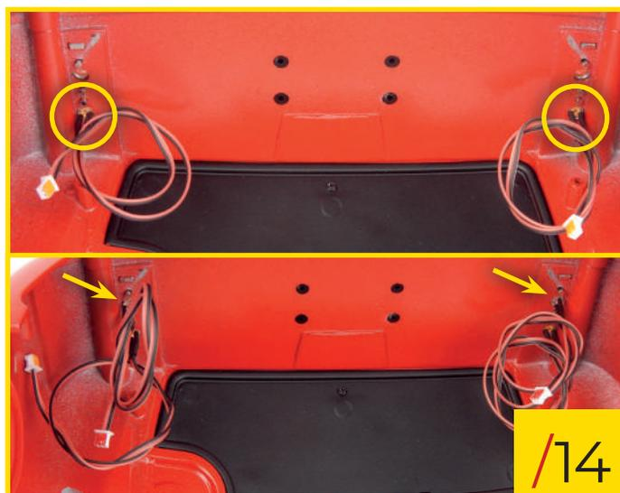
83/14 Insert the LED indicators (orange connector) into their respective slots on the inside of the rear of the body, indicated by the circles in the photo. Now insert the LED brake/rear lights (red connector) into their respective slots, indicated by the arrows.
