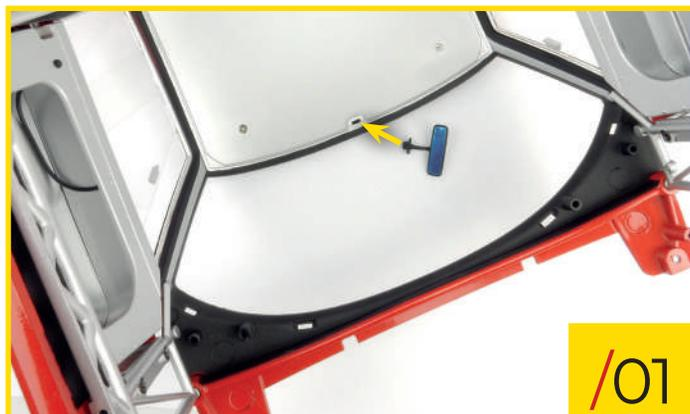
84/01 Install the rear view mirror that you received with stage 79 into its dedicated position on the inside of the roof. Don't remove the blue film for now, it will help protect the surface of the mirror during future assembly sessions.
