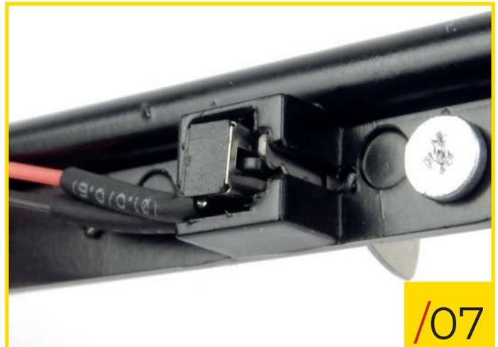
81/07 When your model is complete, inserting the key will turn on the power.
