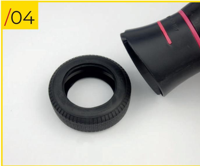
87/04 Before adding the tyre to the rest of the wheel, we recommend that you warm it up slightly (using a hair dryer, for example) to make it more malleable.
