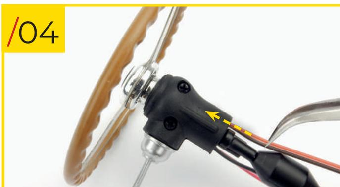
82/04 To avoid damaging the horn cable in the forthcoming assembly steps, we recommend that you push it towards the steering wheel by about 0.5-1 cm.
