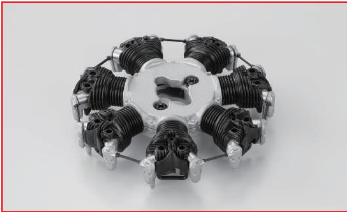
Glue parts 009-03 to each cylinder assembled in stage 08.
