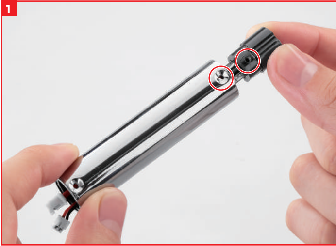
Plug the power connector 085-02 into pipe 085-01 .
