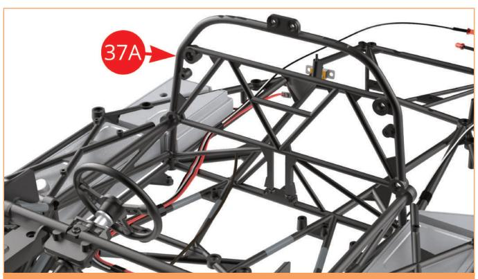
The cockpit partition frame has been installed onto the chassis.
