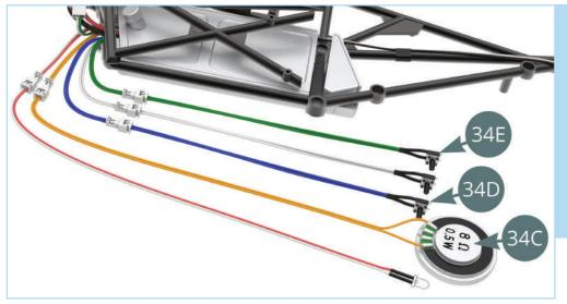
Press the horn switch (green) (34E) – you should hear the sound of the horn through the speaker (34C).
