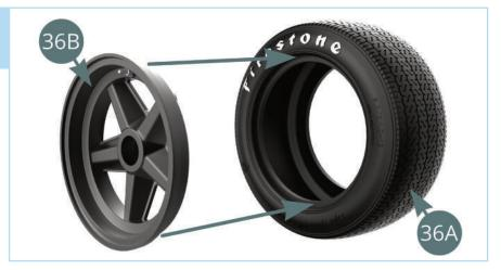
Press the front wheel inner rim (36C) into the front tyre (36A), making sure to align the screw holes with the outer rim (36B). Drive in three BM screws to fix the parts together.
