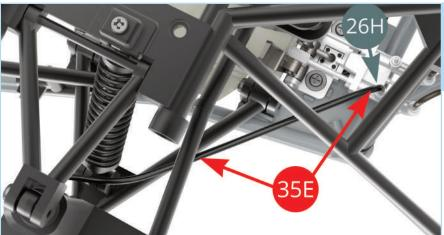
Guide the other end towards the **master cylinder (26H)** and attach it to the closest pin of the cylinder as shown.
