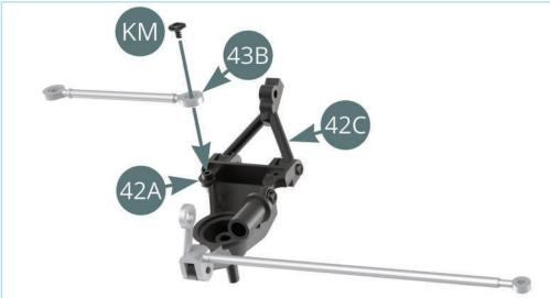
Fit the other **drop link** (43B) onto the rear right upright assembly from Stage 42 and secure with another **KM** screw.
