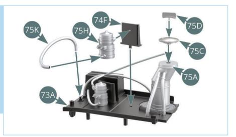
Once assembled, position the right chassis plate (73A) onto the crossbar of the chassis (25A) and the right fuel tank top (33A).
