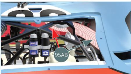
Fit the screw end of the **left pipe (95AB)** to the **left air scoop (82B)** using tweezers.
