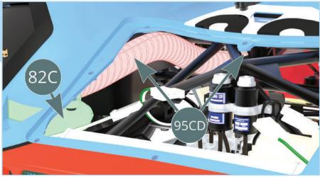
Once the body has been fitted, connect the two ends of the **headlight LED cables (35F)** as shown by the blue arrows. After they are connected, tuck them away from view at the sides (red arrows).
