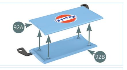
Align the centre spoiler with the **rear hood (90A)** as shown. Fit the holes of the **centre spoiler bottom (92B)** over the indicated screw holes of the rear hood.
