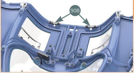
The hinge clamps should look like this once fastened to the front body.
