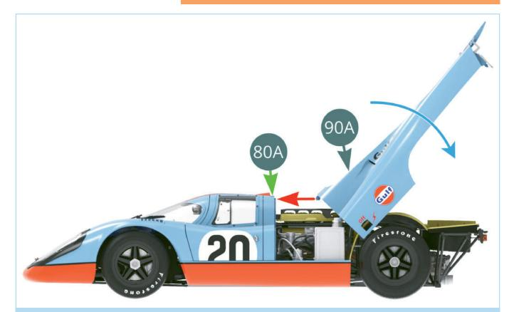
Once the decal is dry, you can fit the rear hood to the model. Remove the transparent tape fitted in Stage 90 if you have not already done so. Align the **rear hood (90A)** with the **front body (80A)** at a 45 degree angle as shown and fit the hood (red arrow). Once in position, lower the hood onto the rear of the model as shown by the blue arrow. Take care not to damage the edges of the front body at the joint (green arrow).
